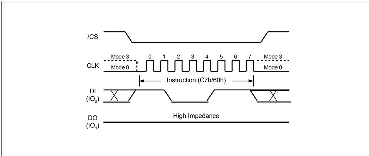
Figure 41. Chip Erase Instruction Sequence Diagram
