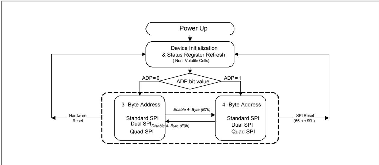
Figure 3. W25Q256JV Serial Flash Memory Operation Diagram
