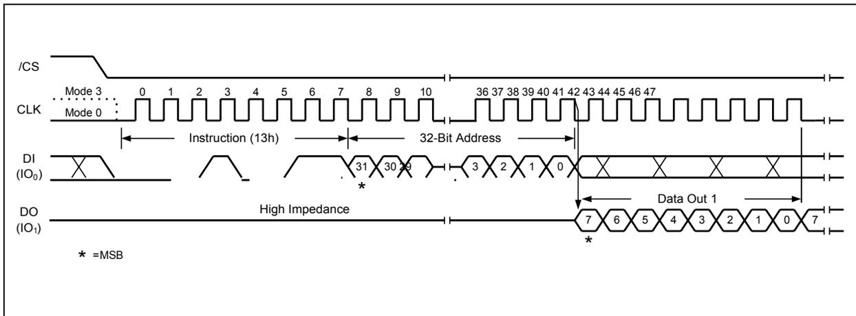
Figure 15. Read Data with 4-Byte Address Instruction
