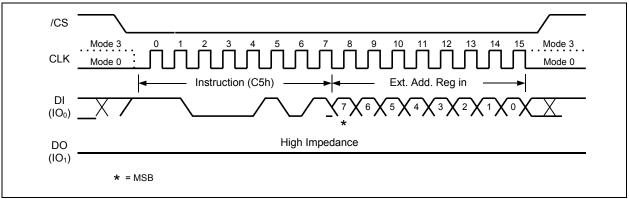
Figure 11. Write Extended Address Register Instruction
