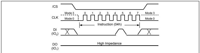
Figure 7. Write Disable Instruction for SPI Mode
