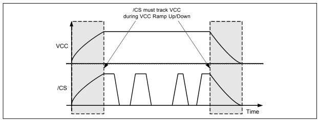
Figure 65b. Power-up, Power-Down Requirement
