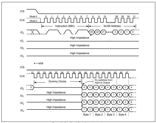
Figure 21. Fast Read Quad Output Instruction
