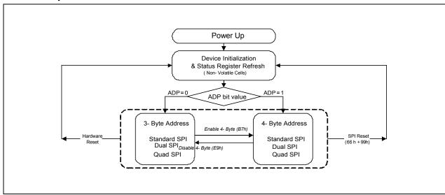
Figure 3. W25Q256JV Serial Flash Memory Operation Diagram
