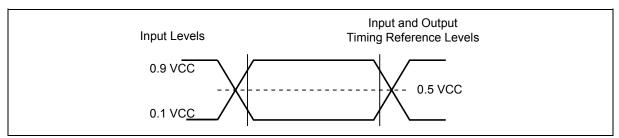
Figure 66. AC Measurement I/O Waveform
