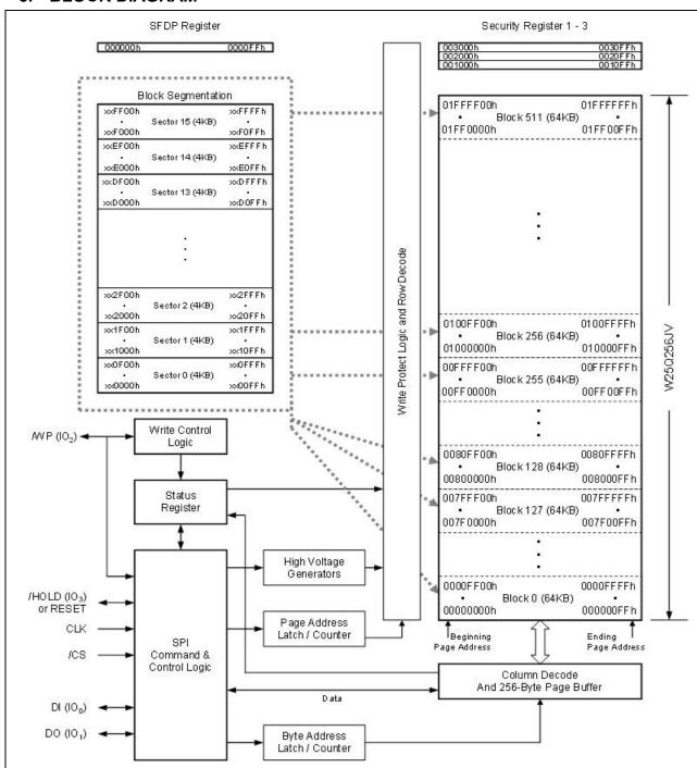
Figure 2. W25Q256JV Serial Flash Memory Block Diagram
