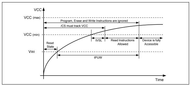
Figure 65a. Power-up Timing and Voltage Levels
