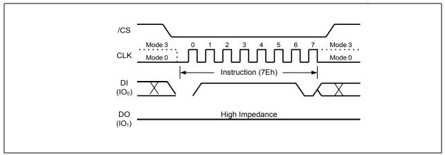
Figure 58. Global Block Lock Instruction for SPI
