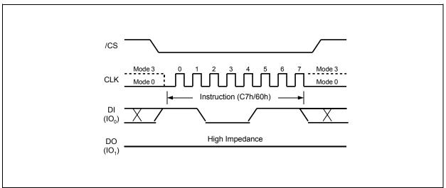
Figure 41. Chip Erase Instruction Sequence Diagram
