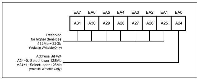
Figure 4e. Extended Address Register
