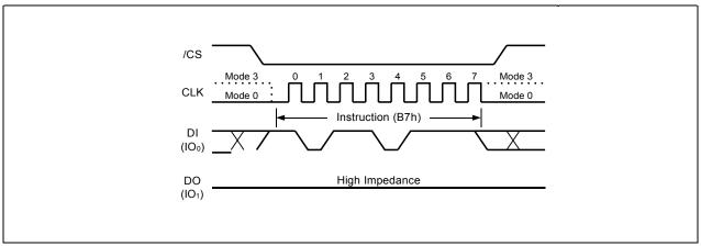
Figure 12. Enter 4-Byte Address Mode instruction
