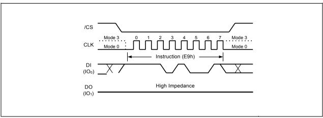
Figure 13. Exit 4-Byte Address Mode instruction
