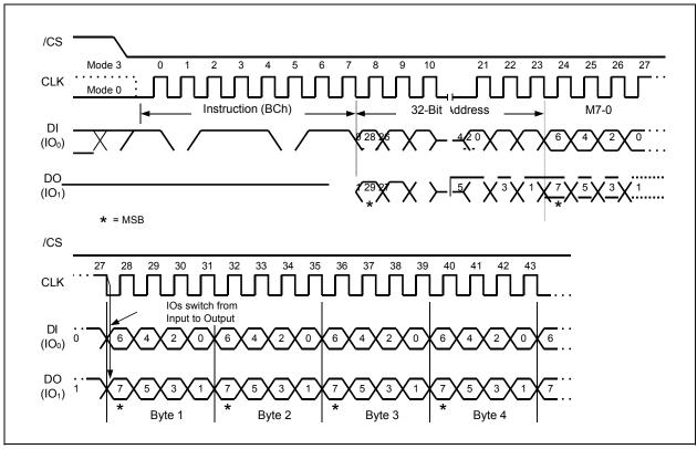
Figure 25a. Fast Read Dual I/O w/ 4-Byte Addr. (M7-M0 shuld set to Fxh, SPI Mode only)
