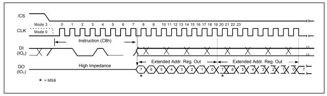
Figure 10a. Read Extended Address Register Instruction
