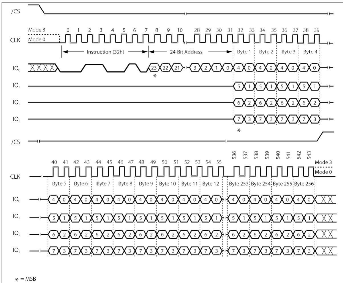
Figure 18. Quad Input Page Program Instruction Sequence Diagram
