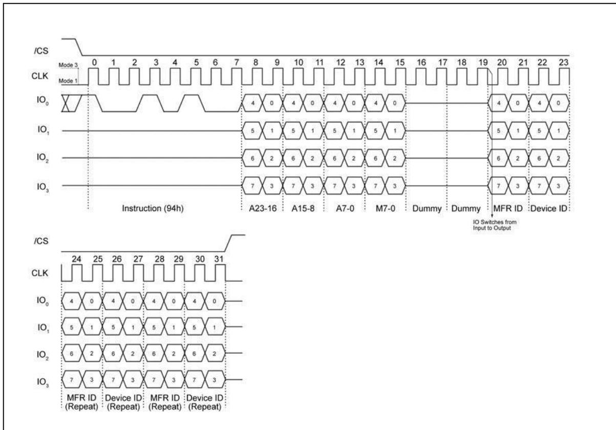
Figure 29. Read Manufacturer / Device ID Quad I/O Diagram
