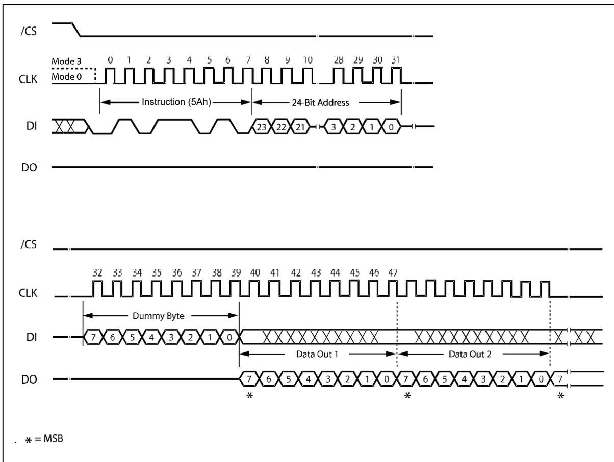
Figure 31b. Read SFDP Register Instruction Sequence Diagram
