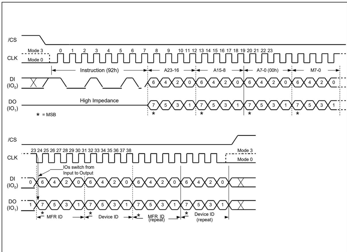
Figure 28. Read Manufacturer / Device ID Dual I/O Diagram
