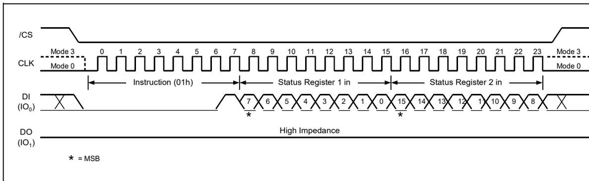
Figure 8. Write Status Register Instruction Sequence Diagram
