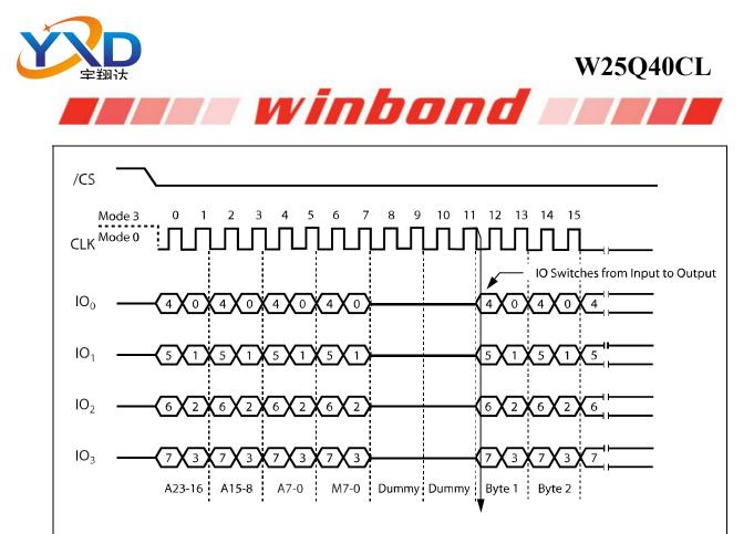
Figure 14b. Fast Read Quad I/O Instruction Sequence (Previous instruction set M5-4 = 10)
