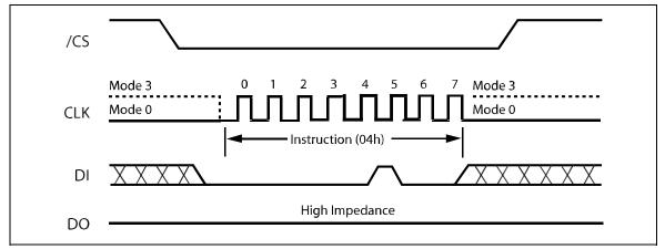
Figure 6. Write Disable Instruction Sequence Diagram
