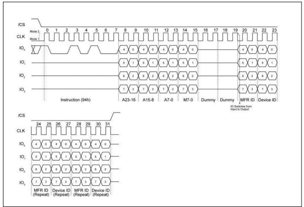
Figure 29. Read Manufacturer / Device ID Quad I/O Diagram
