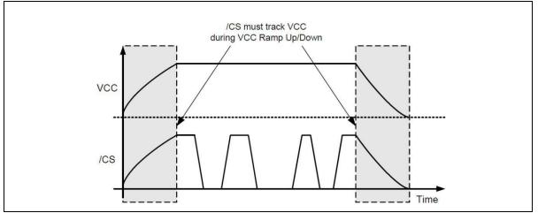
Figure 35b. Power-up, Power-Down Requirement
