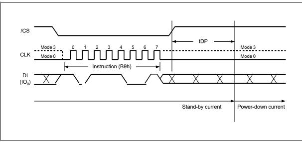
Figure 25. Deep Power-down Instruction Sequence Diagram
