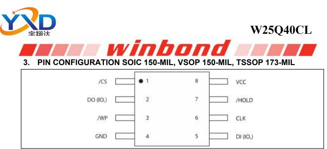
Figure 1a. W25Q40CL Pin Assignments, 8-pin SOIC 150-mil, SOP 208-mil (Package Code SN and SS)
