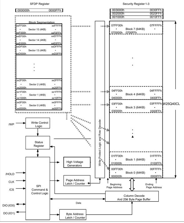
Figure 2. W25Q40CL Serial Flash Memory Block Diagram
