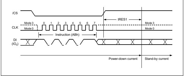
Figure 26a. Release Power-down Instruction Sequence
