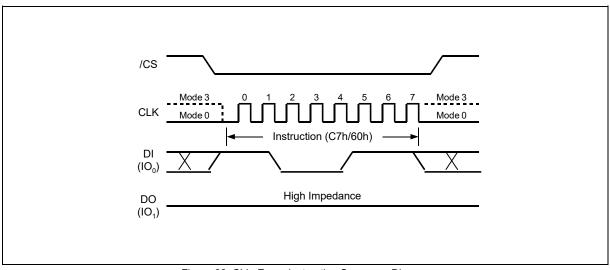
Figure 22. Chip Erase Instruction Sequence Diagram
