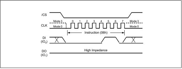
Figure 4. Write Enable Instruction Sequence Diagram
