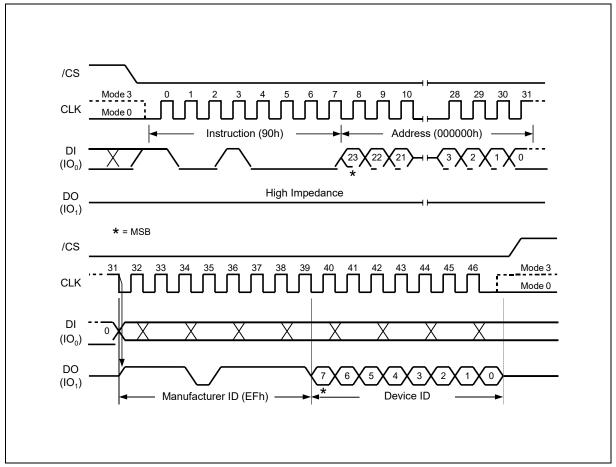
Figure 27. Read Manufacturer / Device ID Diagram
