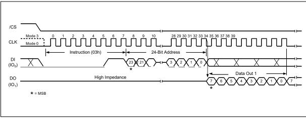
Figure 9. Read Data Instruction Sequence Diagram
