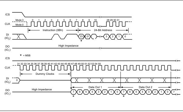
Figure 10. Fast Read Instruction Sequence Diagram
