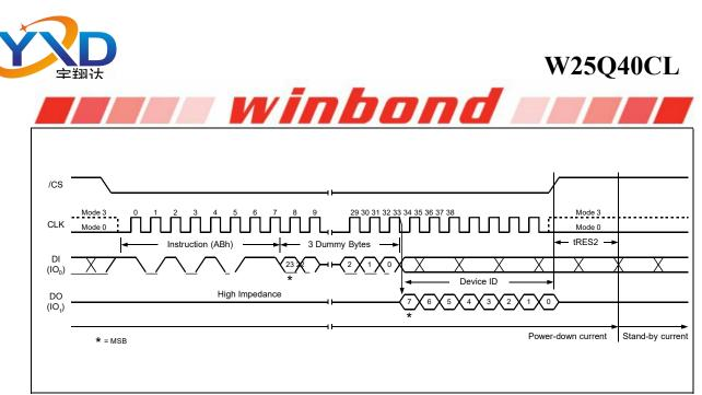
Figure 26b. Release Power-down / Device ID Instruction Sequence Diagram
