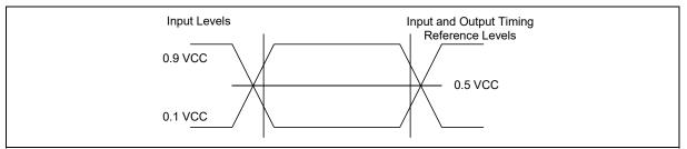
Figure 36. AC Measurement I/O Waveform
