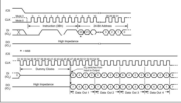
Figure 11. Fast Read Dual Output Instruction Sequence Diagram
