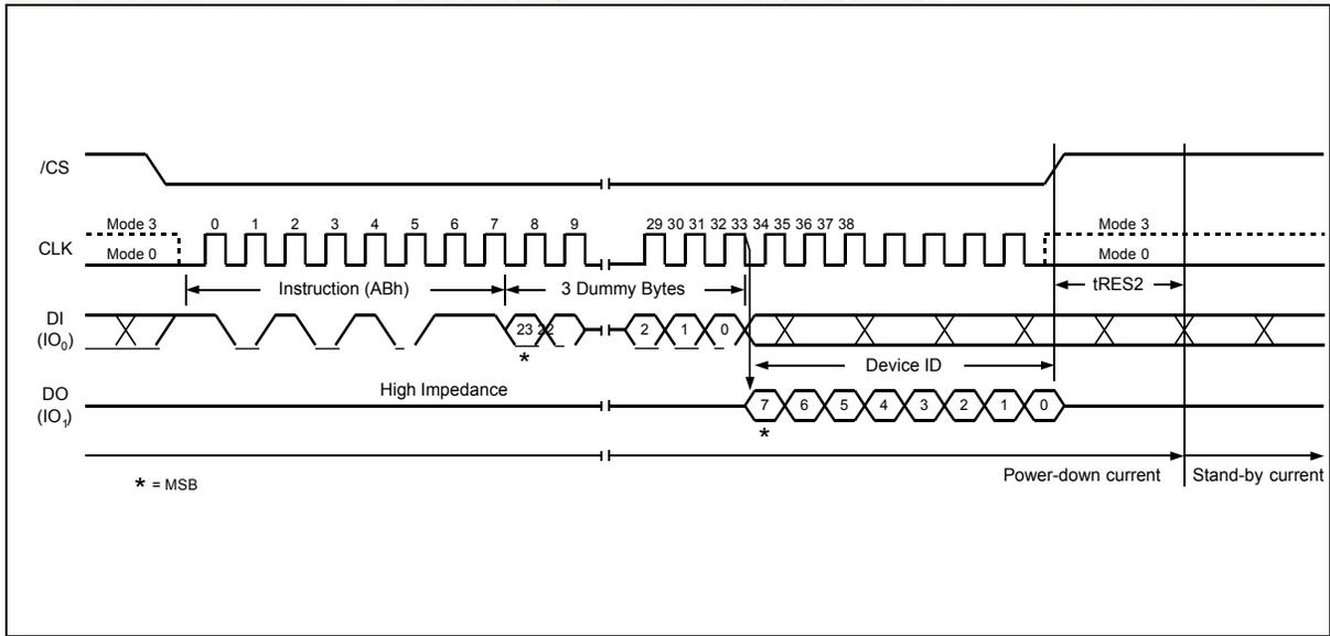
Figure 21. Release Power-down / Device ID Instruction Sequence Diagram
