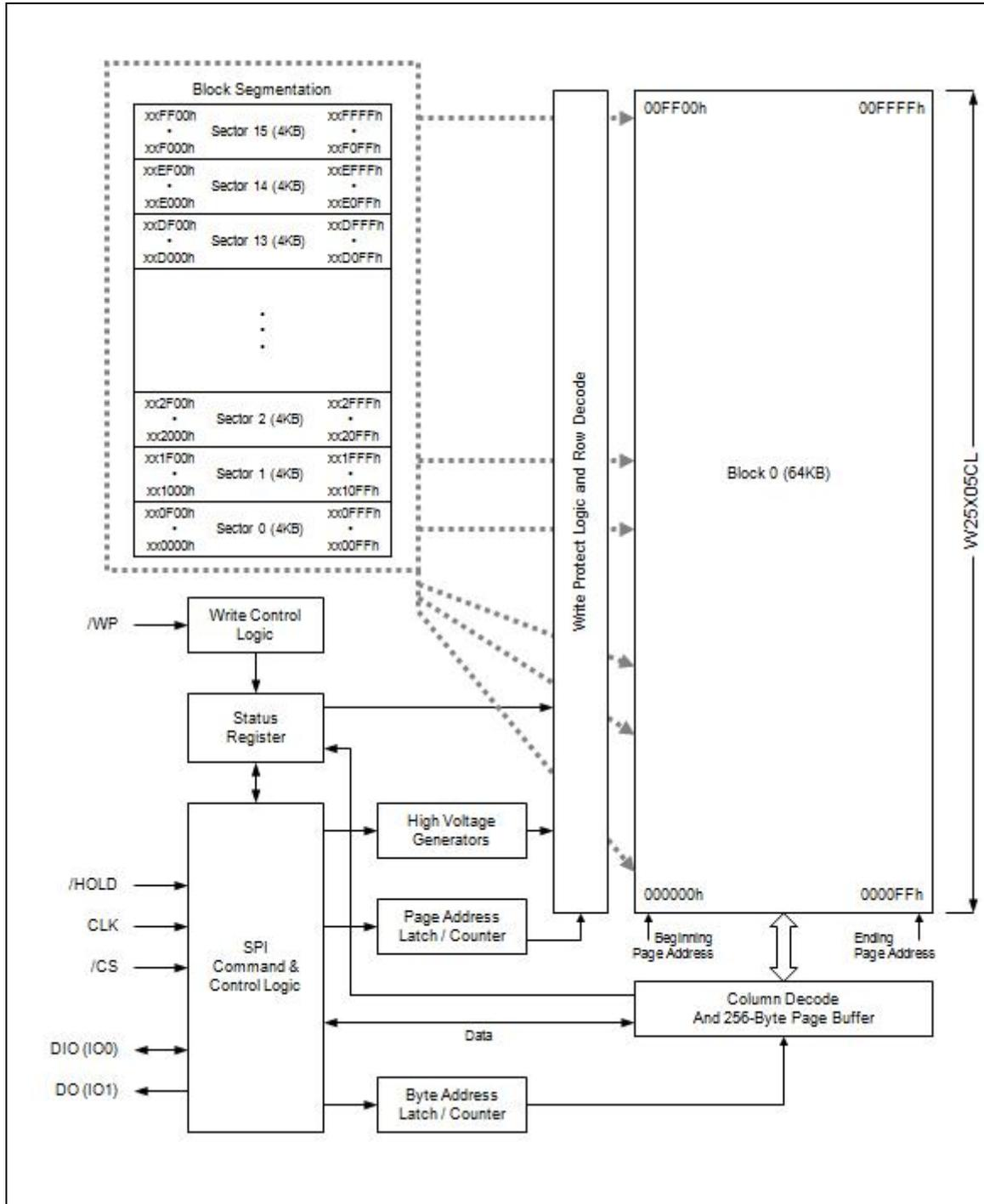
Figure 2. W25X05CL Serial Flash Memory Block Diagram
