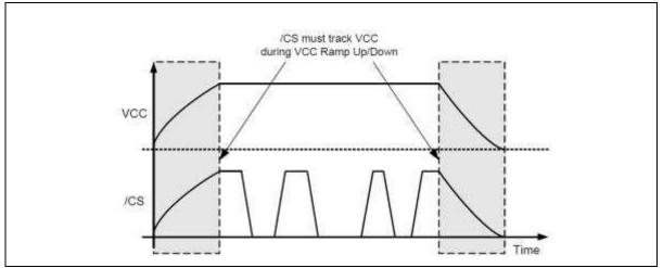
Figure 26b. Power-up, Power-Down Requirement
