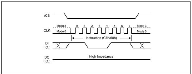
Figure 18. Chip Erase Instruction Sequence Diagram
