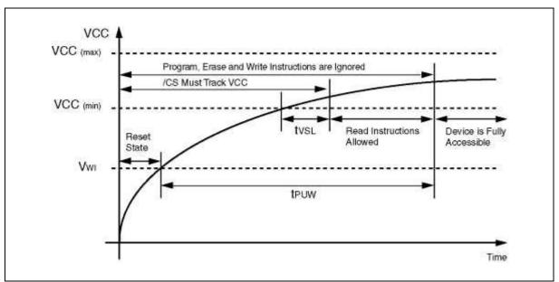
Figure 26a. Power-up Timing and Voltage Levels
