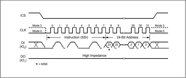
Figure 16. 32KB Block Erase Instruction Sequence Diagram
