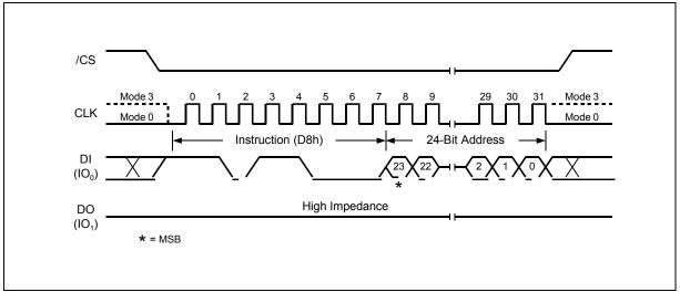
Figure 17. Block Erase Instruction Sequence Diagram
