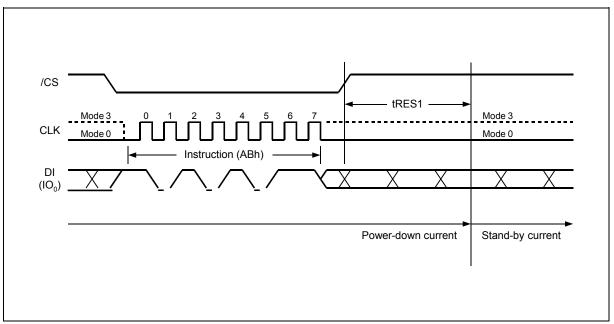
Figure 20. Release Power-down Instruction Sequence
