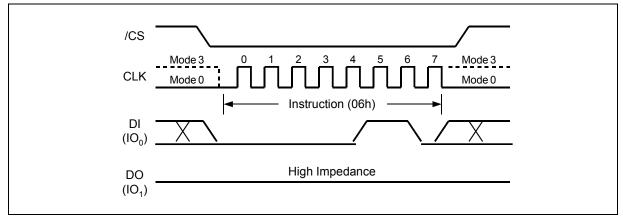
Figure 4. Write Enable Instruction Sequence Diagram
