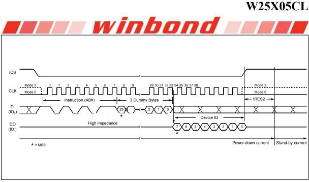
Figure 21. Release Power-down / Device ID Instruction Sequence Diagram
