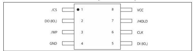
Figure 1a. W25X05CL Pin Assignments, 8-pin SOIC 150-mil, VSOP 150-mil and TSSOP8 173-mil (Package Code SN, SV and SD)
