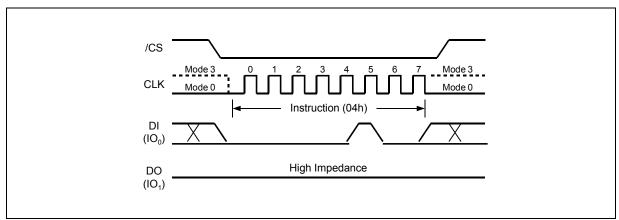
Figure 6. Write Disable Instruction Sequence Diagram
