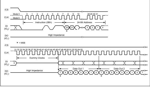
Figure 10. Fast Read Instruction Sequence Diagram
