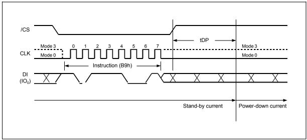
Figure 19. Deep Power-down Instruction Sequence Diagram
