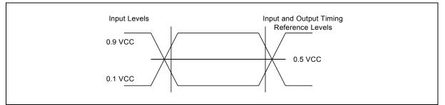
Figure 27. AC Measurement I/O Waveform
