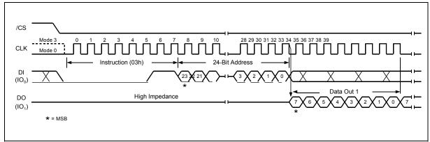
Figure 9. Read Data Instruction Sequence Diagram
