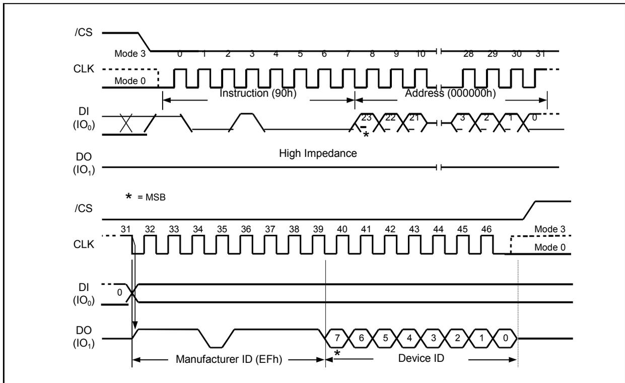
Figure 39. Read Manufacturer / Device ID Instruction (SPI Mode)
