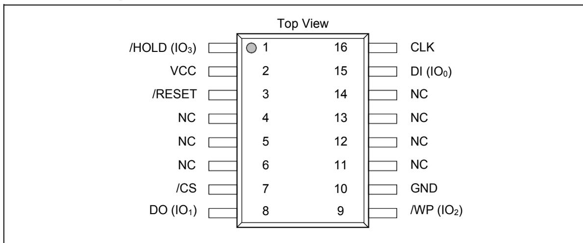
Figure 1c. W25Q128FV Pin Assignments, 16-pin SOIC 300-mil (Package Code F)
