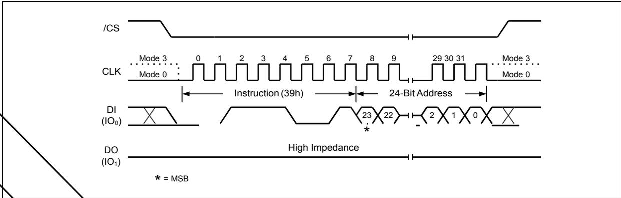
Figure 53a. Individual Block Unlock Instruction (SPI Mode)
