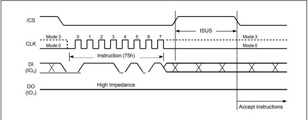
Figure 35a. Erase/Program Suspend Instruction (SPI Mode)
