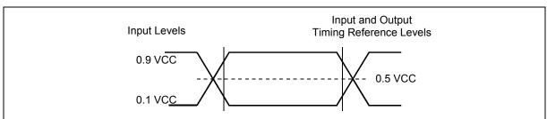
Figure 59. AC Measurement I/O Waveform
