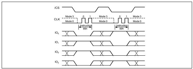
Figure 57b. Enable Reset and Reset Instruction Sequence (QPIMode)
