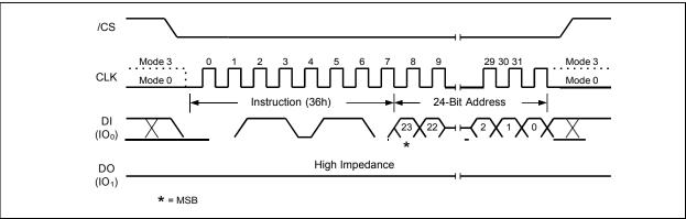
Figure 52a. Individual Block/Sector Lock Instruction (SPI Mode)
