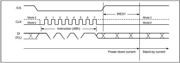
Figure 38a. Release Power-down Instruction (SPI Mode)
