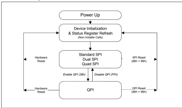
Figure 3. W25Q128FV Serial Flash Memory Operation Diagram
