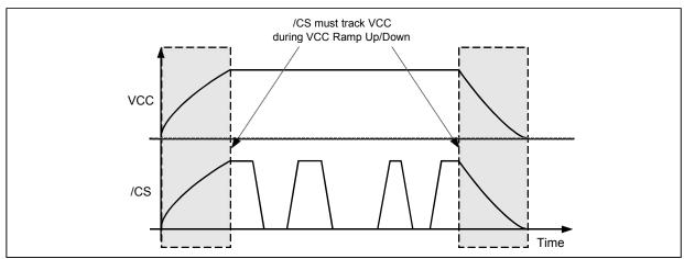
Figure 58b. Power-up, Power-DownRequirement
