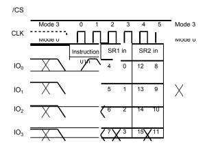
Figure 9d. Write Status Register-1/2 Instruction (QPI Mode)
