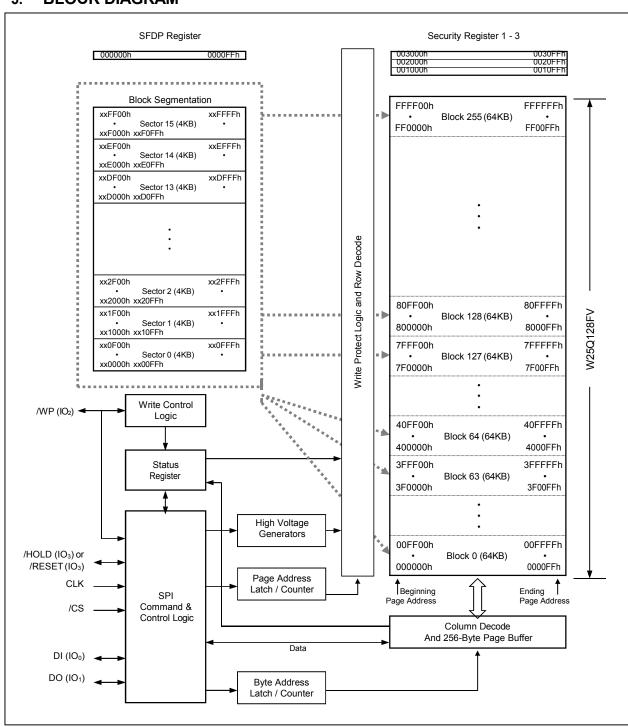
Figure 2. W25Q128FV Serial Flash Memory Block Diagram
