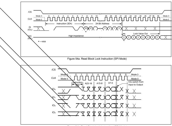
Figure 54b. Read Block Lock Instruction (QPI Mode)
