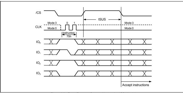
Figure 35b. Erase/Program Suspend Instruction (QPI Mode)
