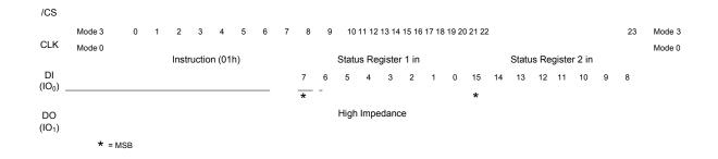
Figure 9c. Write Status Register-1/2 Instruction (SPI Mode)
