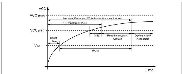
Figure 58a. Power-up Timing and Voltage Levels
