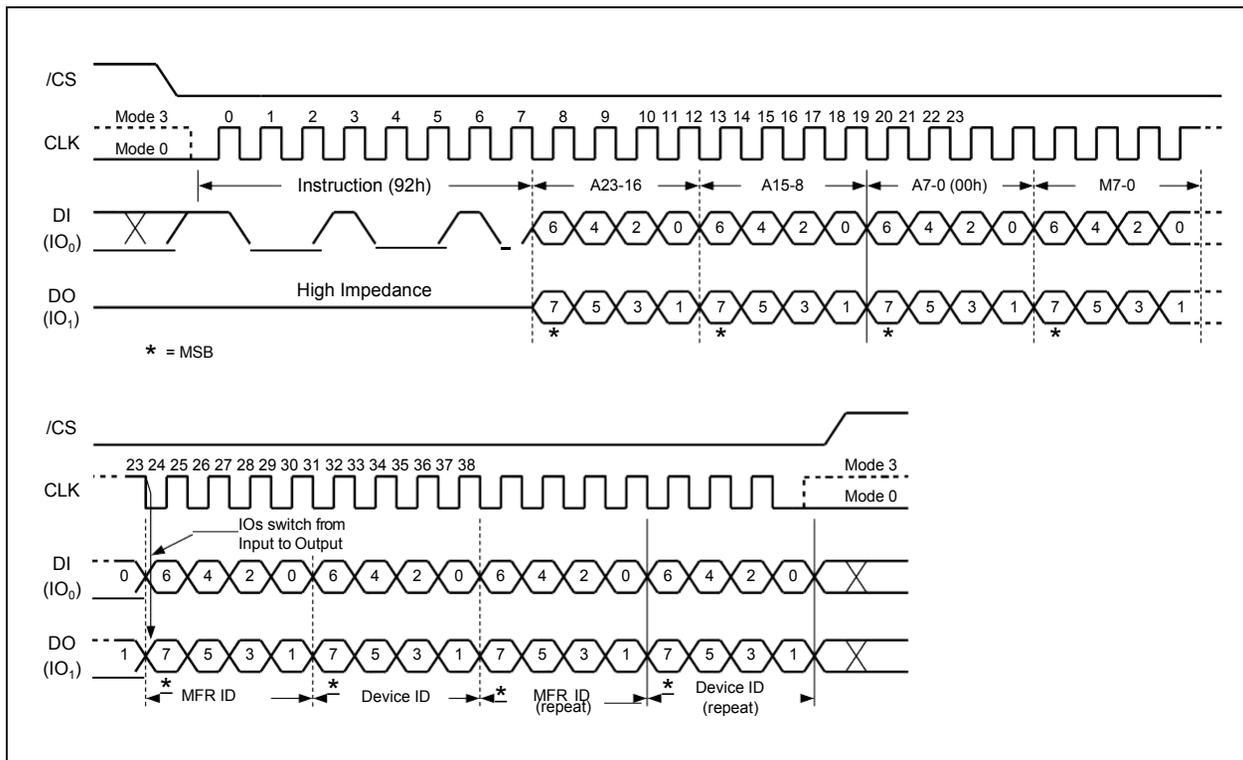
Figure 40. Read Manufacturer / Device ID Dual I/O Instruction
