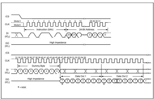
Figure 44. Read SFDP Register Instruction Sequence Diagram
