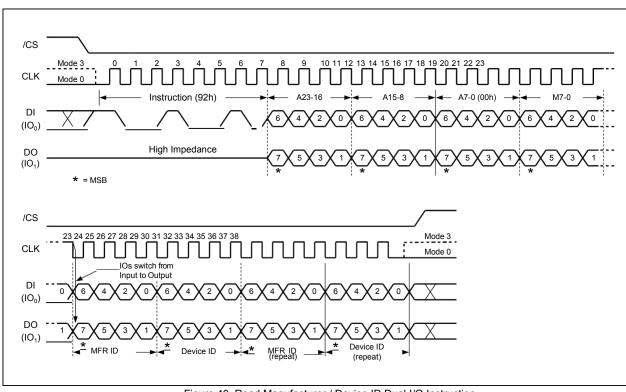
Figure 40. Read Manufacturer / Device ID Dual I/O Instruction
