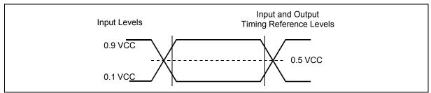
Figure 59. AC Measurement I/O Waveform
