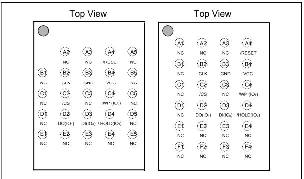
Figure 1d. W25Q64JV Ball Assignments, 24-ball TFBGA 8x6-mm (Package Code TB/TC)
