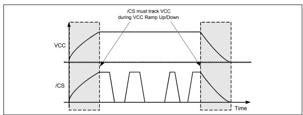
Figure 58b. Power-up, Power-Down Requirement
