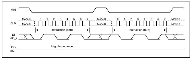
Figure 58. Enable Reset and Reset Instruction Sequence
