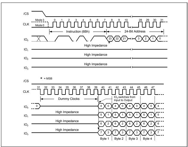
Figure 20. Fast Read Quad Output Instruction
