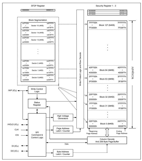
Figure 2. W25Q64JV Serial Flash Memory Block Diagram
