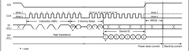
Figure 38c. Release Power-down / Device ID Instruction
