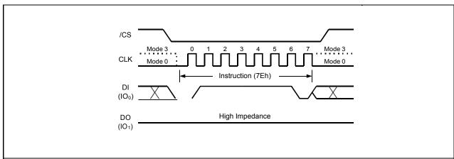
Figure 56. Global Block Lock Instruction for SPI Mode
