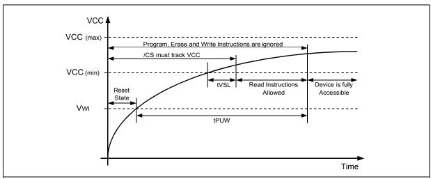
Figure 58a. Power-up Timing and Voltage Levels
