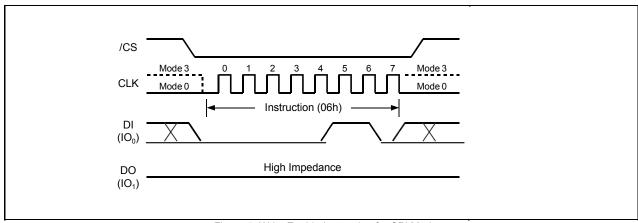
Figure 5. Write Enable Instruction for SPI Mode
