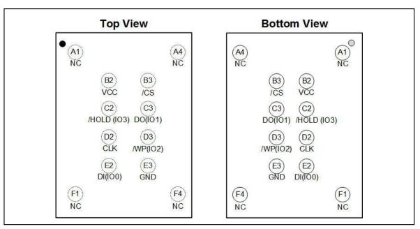
Figure 1e. W25Q64JV Ball Assignments, 12-ball WLCSP (Package Code BY)
