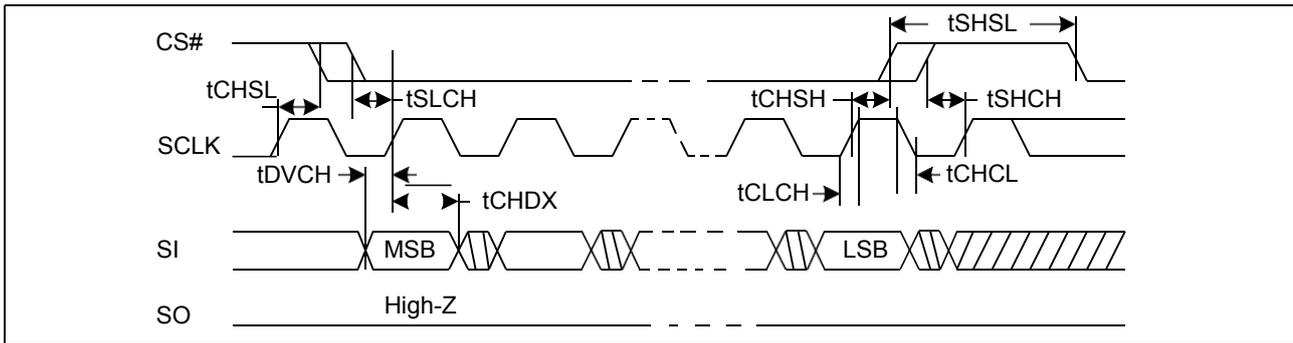
Figure 44. Output Timing
