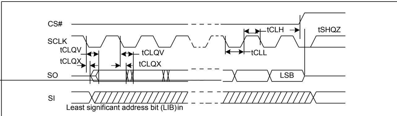
Figure 45. Resume to Suspend Timing Diagram
