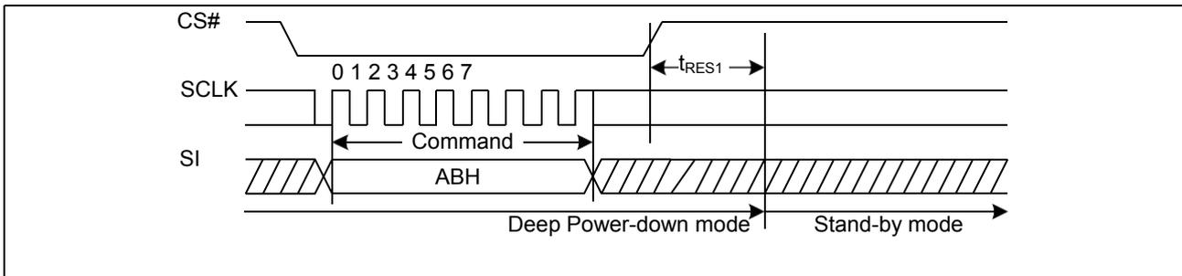
**Figure 27. Release Power-Down/Read Device ID Sequence Diagram**
