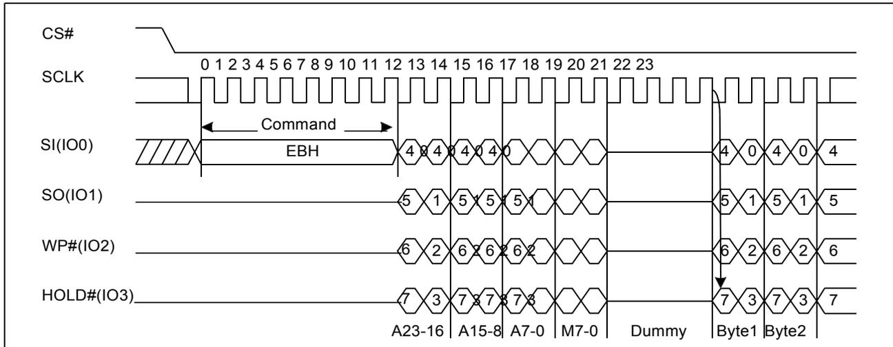
**Figure 14. Quad I/O Fast Read Sequence Diagram (M5-4= (1, 0))**
