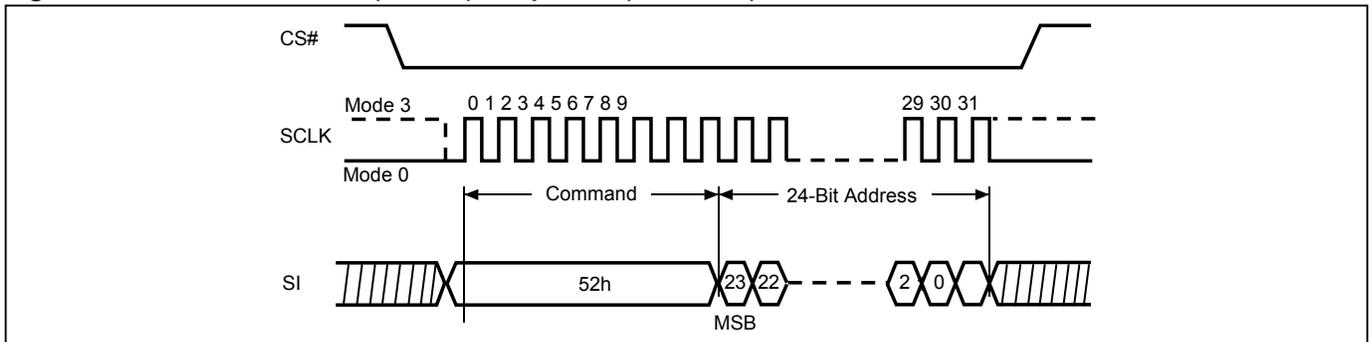
**Figure 46. Block Erase 32KB (BE32K) Sequence (QPI Mode)**
