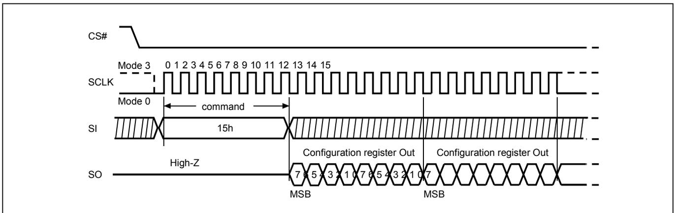
**Figure 19. Read Configuration Register (RDCR) Sequence (QPI Mode)**
