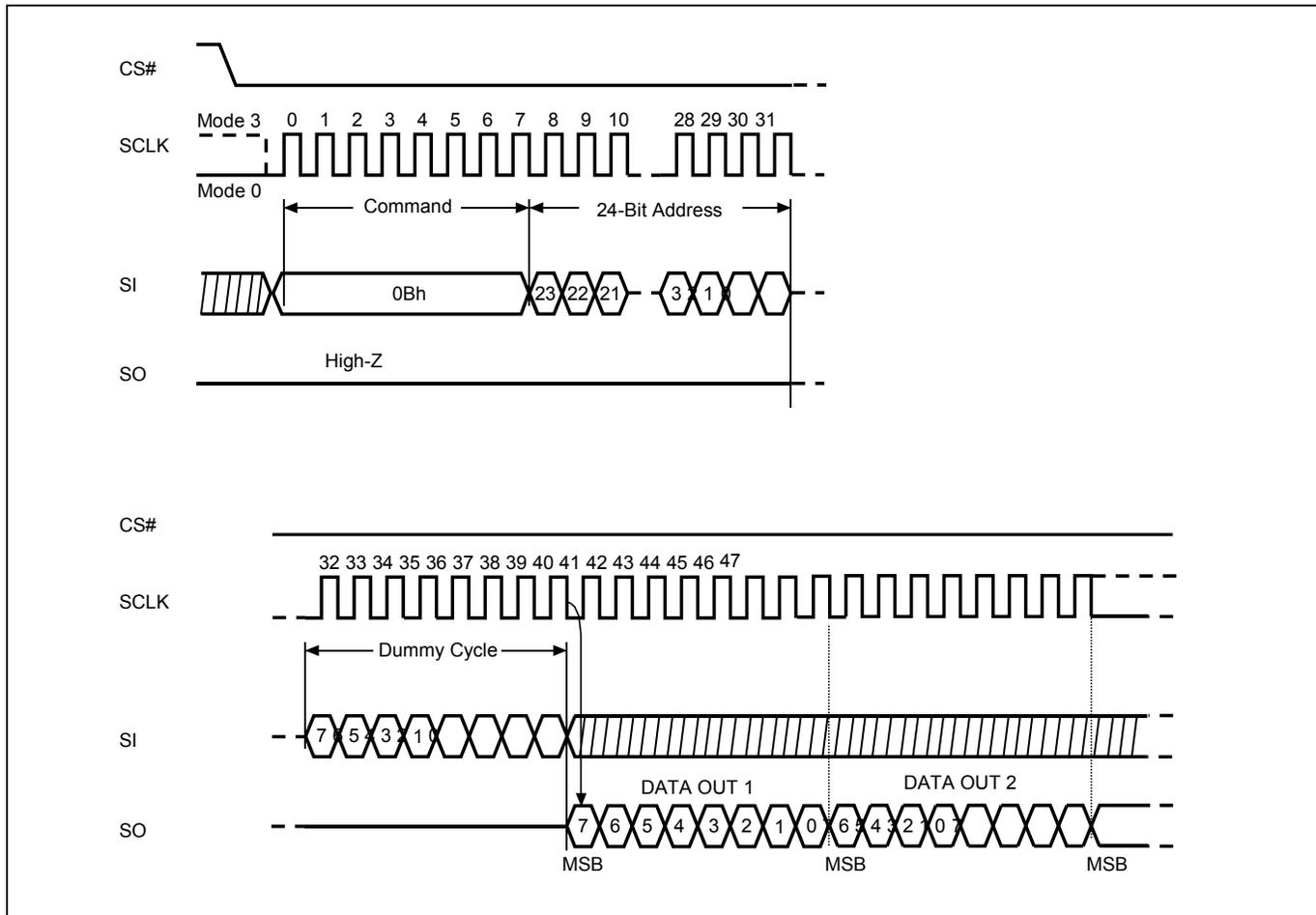
**Figure 28. Read at Higher Speed (FAST\_READ) Sequence (QPI Mode)**
