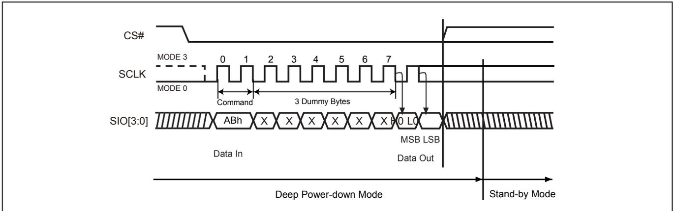
**Figure 13. Release from Deep Power-down (RDP) Sequence (SPI Mode)**
