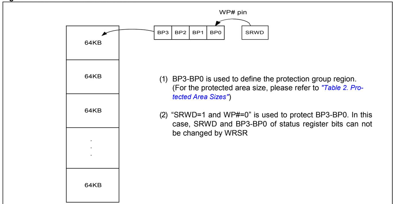
**Figure 58. The individual block lock mode is effective after setting WPSEL=1**
