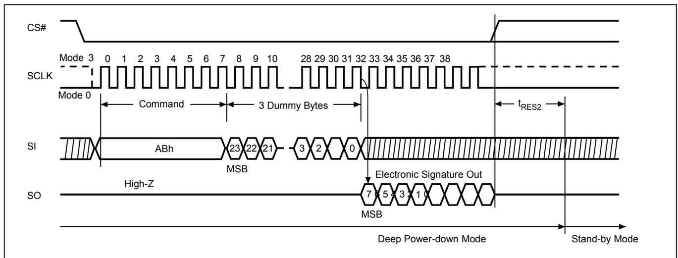
**Figure 12. Read Electronic Signature (RES) Sequence (QPI Mode)**
