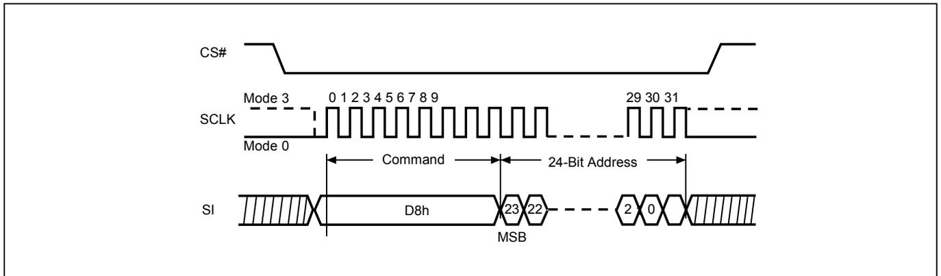
**Figure 48. Block Erase (BE) Sequence (QPI Mode)**
