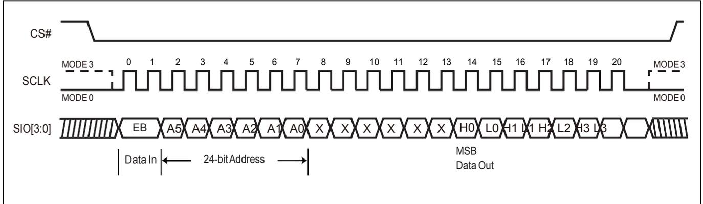
**Figure 35. 4 x I/O Read Mode Sequence (QPI Mode), for MX25U12835FZNI-08G only**
