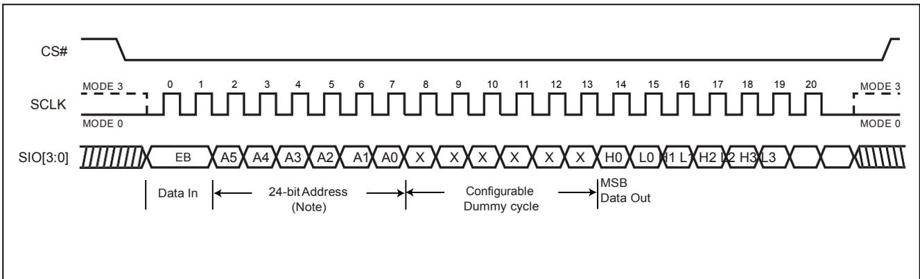
**Note:** The Configurable Dummy Cycle (default = 6) is set by Configuration Register Bit. Please check ["Dummy Cycle and Frequency Table"](#) for details.
