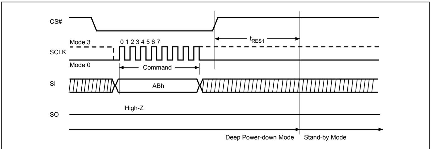
**Figure 14. Release from Deep Power-down (RDP) Sequence (QPI Mode)**
