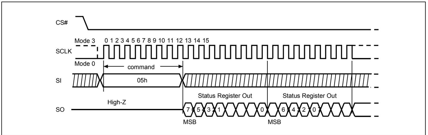
**Figure 17. Read Status Register (RDSR) Sequence (QPI Mode)**
