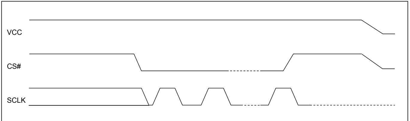
**Figure 79. Power-up Timing**
