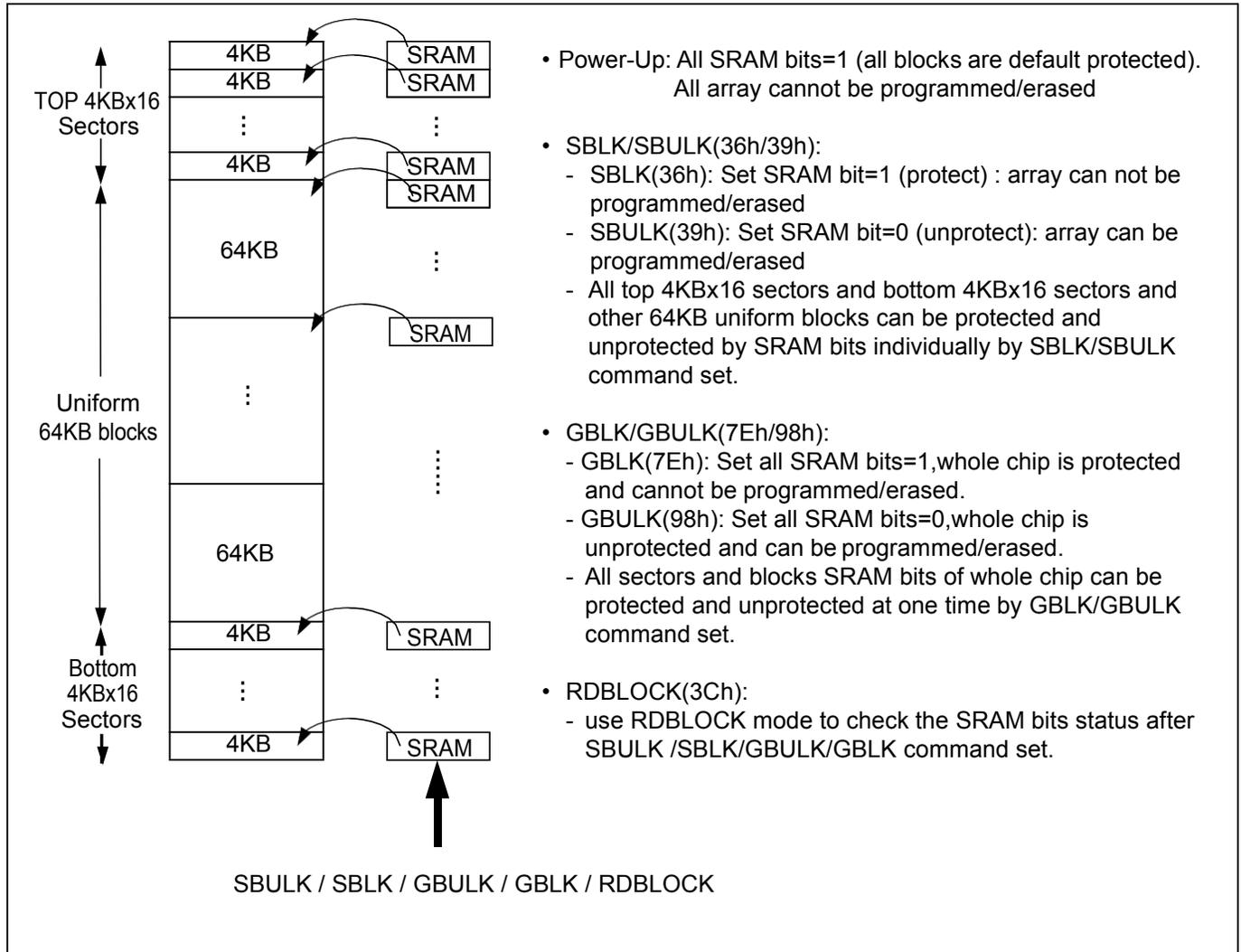
**Figure 59. Write Protection Selection (WPSEL) Sequence (Command 68)**
