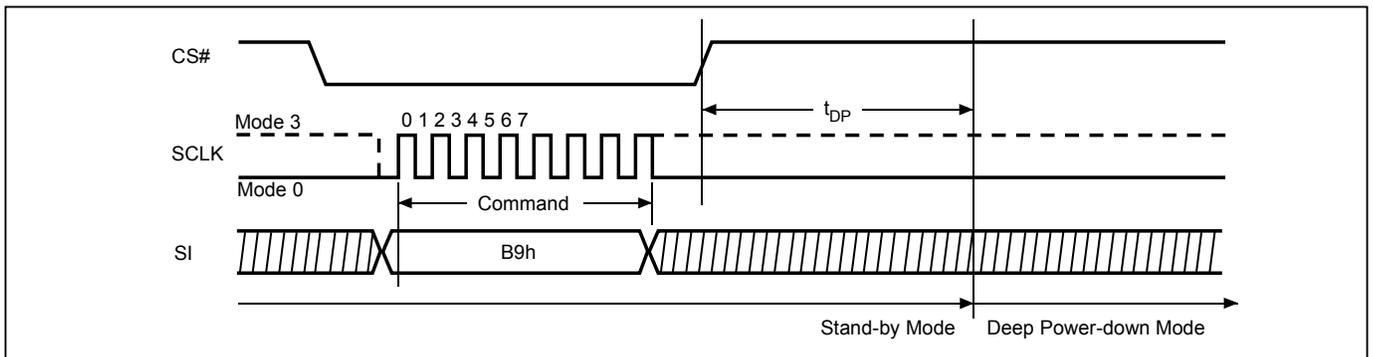
**Figure 55. Deep Power-down (DP) Sequence (QPI Mode)**
