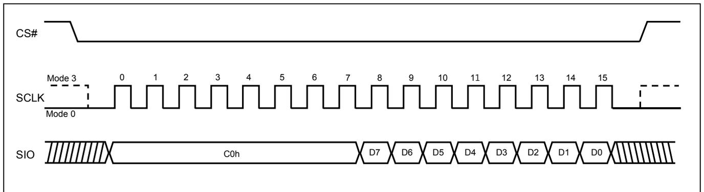
**Figure 38. Burst Read (QPI Mode)**
