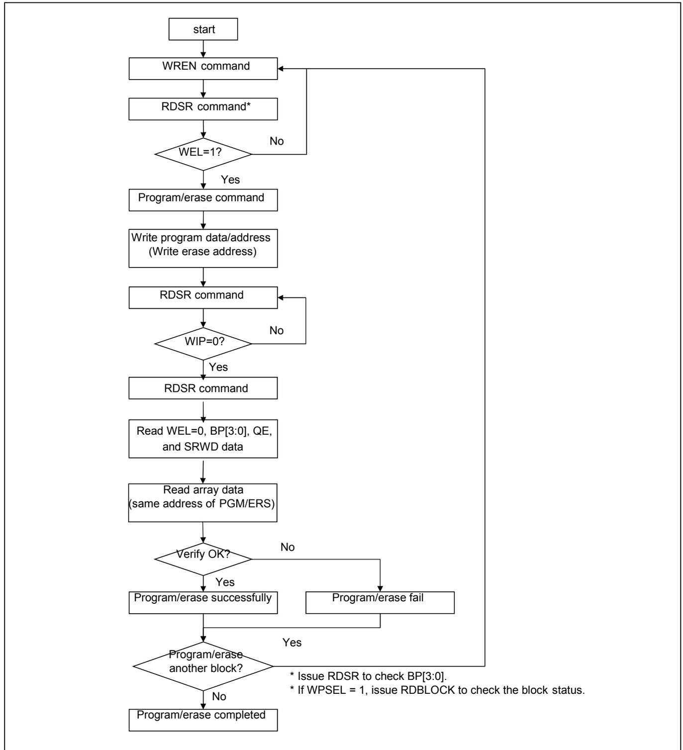
Figure 21. Program/Erase flow without read array data (read P\_FAIL/E\_FAIL flag)
