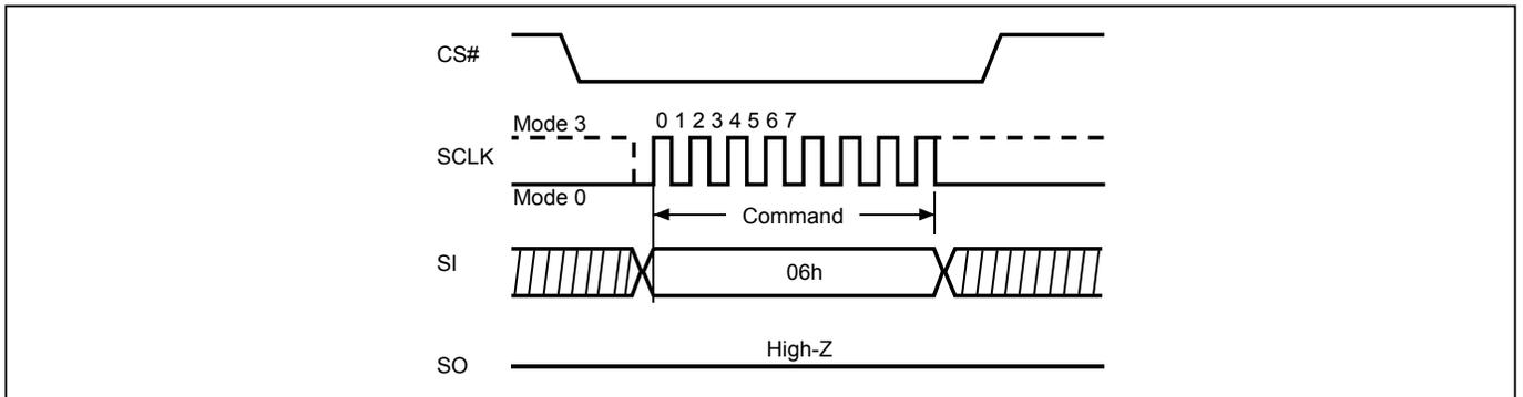
**Figure 7. Write Enable (WREN) Sequence (QPI Mode)**
