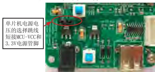
单片机电源电压的选择跳线短接MCU-VCC和5V电源管脚
