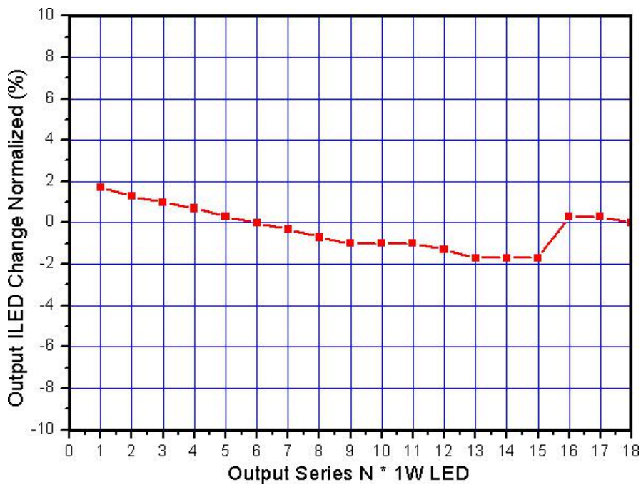
Figure6. Output ILED Load Regulation VS Output N*1W LED
