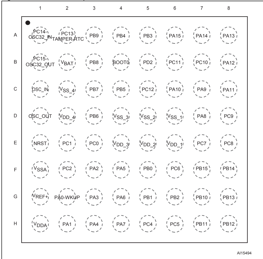
Figure 6. STM32F103xx performance line TFBGA64 ballout
