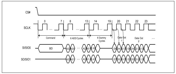
**Note:** SI/SIO0 or SO/SIO1 should be kept "0h" or "Fh" in the first two dummy cycles. In other words, P2=P0 or P3=P1 is necessary.
