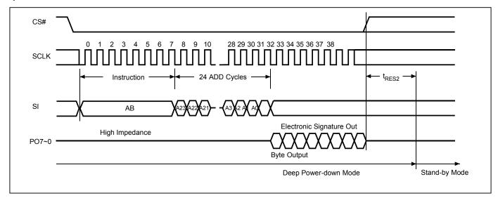
**Note:** Under parallel mode, the fastest access clock freg. will be changed to 6MHz(SCLK pin clock freg.) To release from Deep Power-down mode and read ID in parallel mode, which requires a parallel mode command (55h) before the read status register command.
