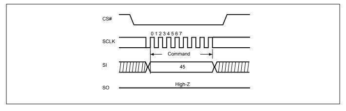
Figure 31-3. Parallel Mode Read Identification (Parallel RDID) Sequence (Command 9F)
