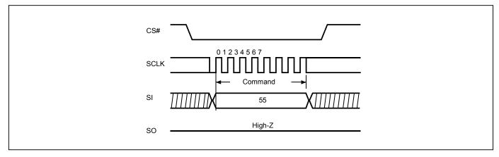
Figure 31-2. Exit Parallel Mode (EXPLM) Sequence (Command 45)
