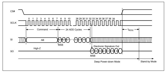
Figure 33. Read Electronic Signature (RES) Sequence (Command AB)
