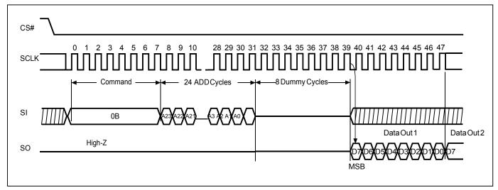
Figure 18. Fast DT Read (FASTDTRD) Sequence (Command 0D)
