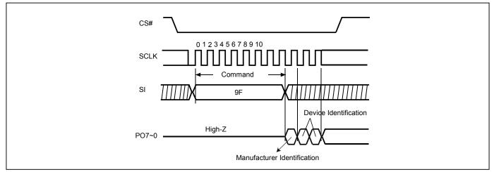
**Note:** There are 3 data bytes which would be output sequentially for Manufacturer and Device ID 1'st byte (Memory Type) and Device ID 2'nd byte (Memory Density).
