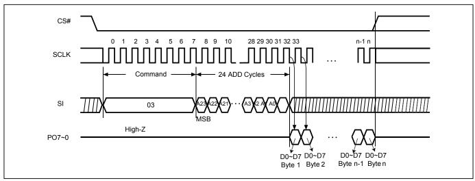
Figure 31-6. Parallel Mode Read Array (Parallel READ) Sequence (Command 03)
