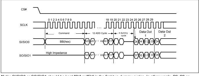
**Note:** SI/SIO0 or SO/SIO1 should be kept "0h" or "Fh" in the first two dummy cycles. In other words, P2=P0 or P3=P1 is necessary.
