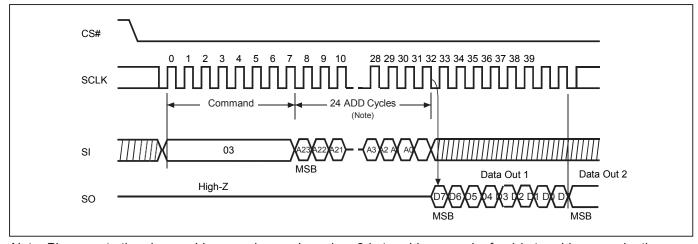
Note: Please note the above address cycles are based on 3-byte address mode, for 4-byte address mode, the address cycles will be increased.
