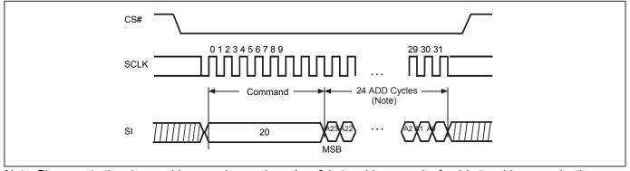
Note: Please note the above address cycles are based on 3-byte address mode, for 4-byte address mode, the address cycles will be increased.
