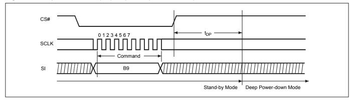
Figure 29. Read Electronic Signature (RES) Sequence (Command AB)
