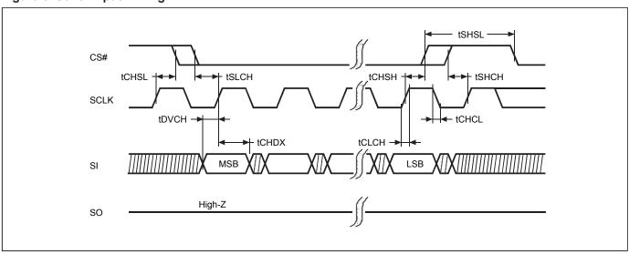
Figure 7. Output Timing
