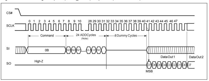
Note: Please note the above address cycles are based on 3-byte address mode, for 4-byte address mode, the address cycles will be increased.
