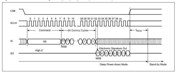
Figure 30. Release from Deep Power-down (RDP) Sequence (Command AB)
