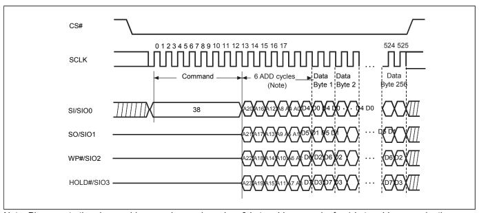
Note: Please note the above address cycles are based on 3-byte address mode, for 4-byte address mode, the address cycles will be increased.
