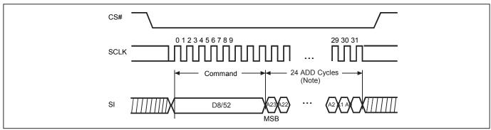
Note: Please note the above address cycles are based on 3-byte address mode, for 4-byte address mode, the address cycles will be increased.
