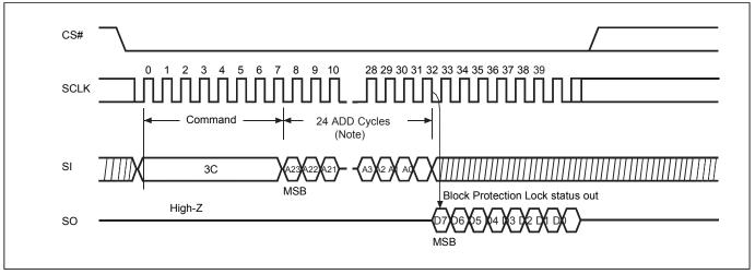
Note: Please note the above address cycles are based on 3-byte address mode, for 4-byte address mode, the address cycles will be increased.
