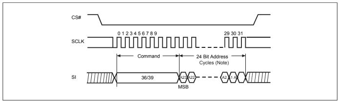
Note: Please note the above address cycles are based on 3-byte address mode, for 4-byte address mode, the address cycles will be increased.
