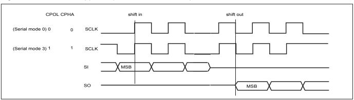
Figure 1. Serial Modes Supported (for Normal Serial mode)
