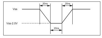
Figure 4. Maximum Positive Overshoot Waveform
