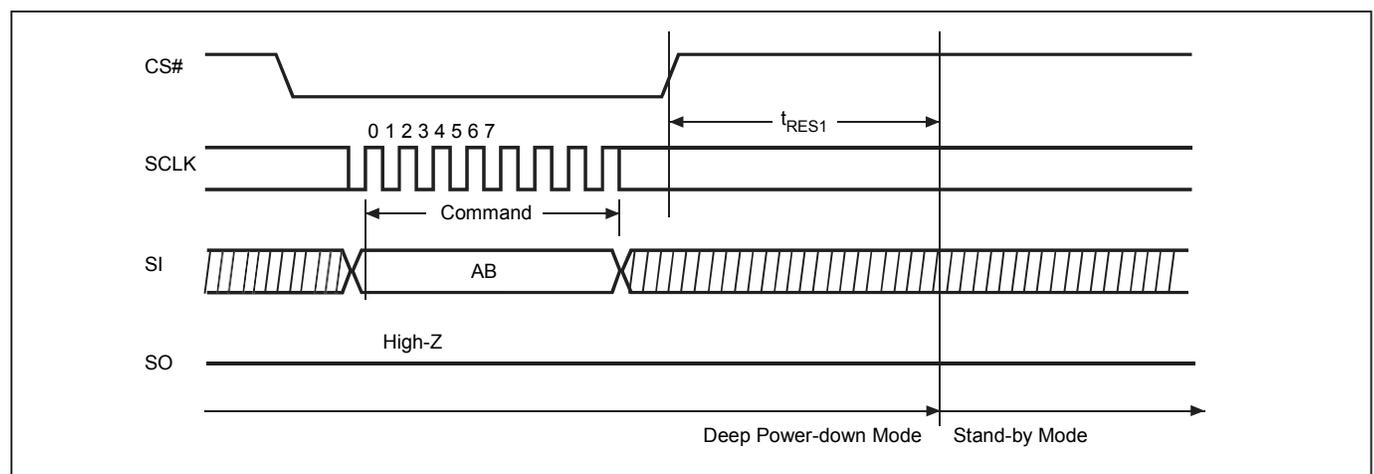
**Figure 31. Read Electronic Manufacturer & Device ID (REMS) Sequence (Command 90 or EF or DF)**
