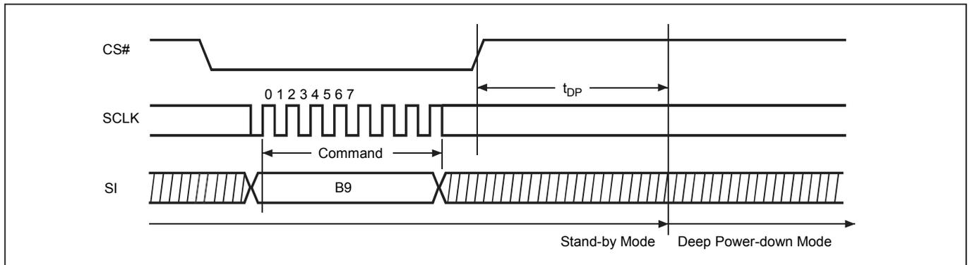
**Figure 29. Read Electronic Signature (RES) Sequence (Command AB)**
