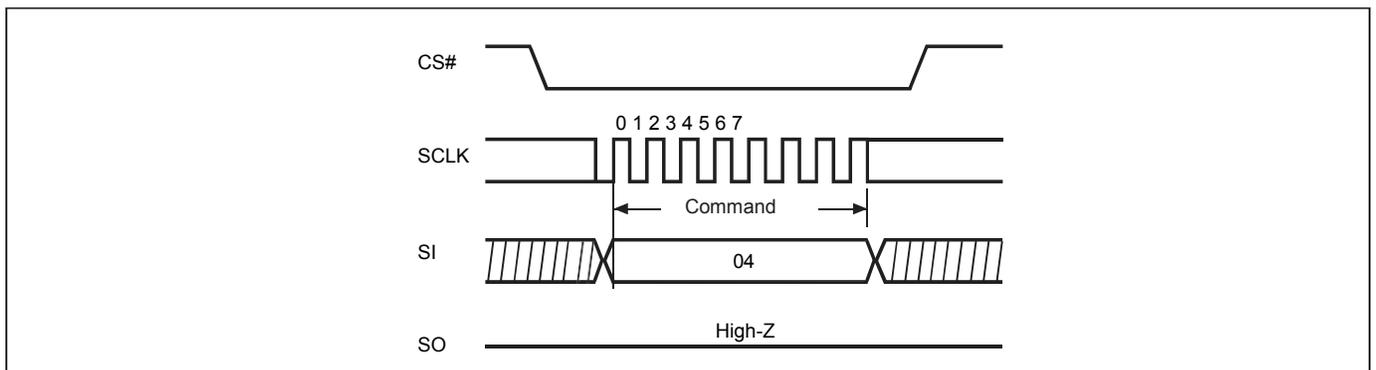
**Figure 12. Read Identification (RDID) Sequence (Command 9F)**
