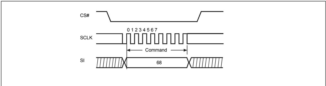
**Figure 33. Single Block Lock/Unlock Protection (SBLK/SBULK) Sequence (Command 36/39)**
