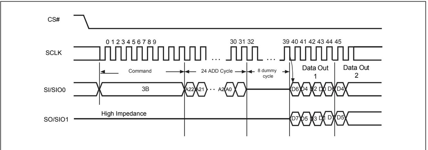
**Figure 19. 4 x I/O Read Mode Sequence (Command EB)**
