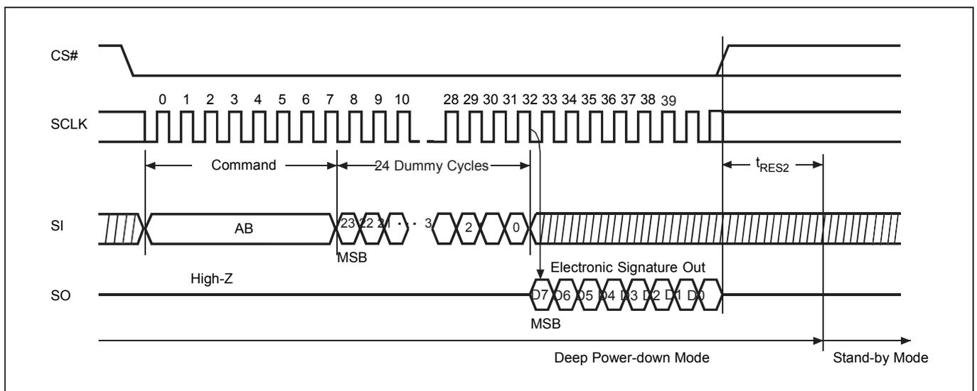
**Figure 30. Release from Deep Power-down (RDP) Sequence (Command AB)**
