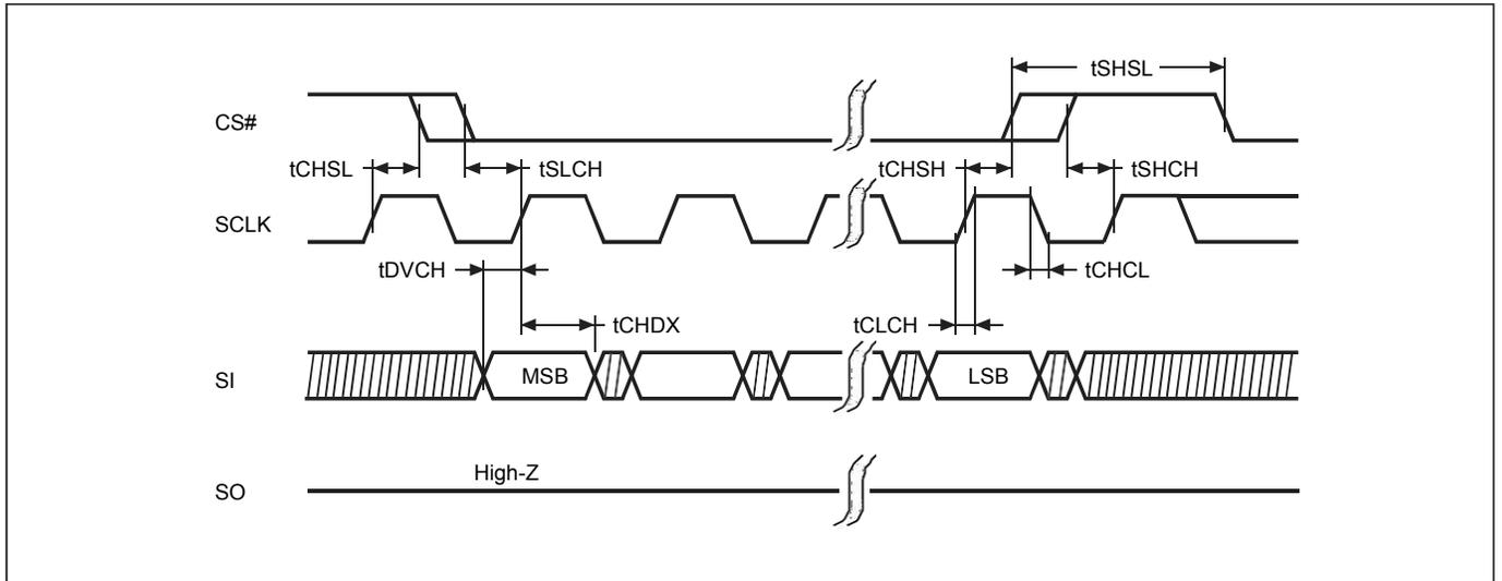
**Figure 7. Output Timing**
