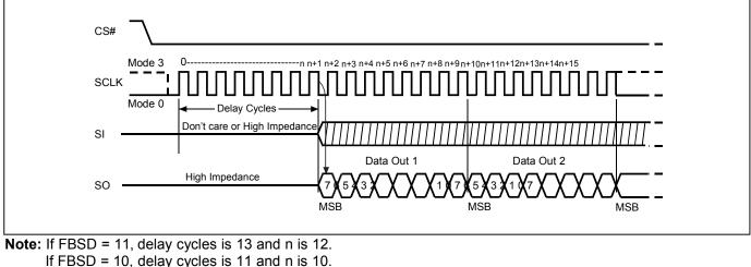
If FBSD = 10, delay cycles is 11 and n is 10. If FBSD = 01, delay cycles is 9 and n is 8. If FBSD = 00, delay cycles is 7 and n is 6.
