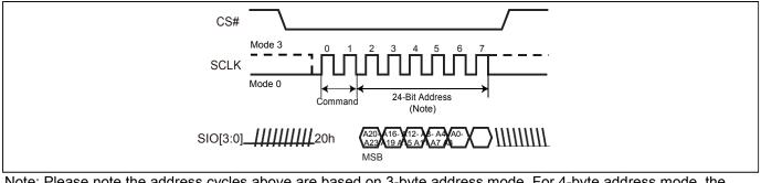
Note: Please note the address cycles above are based on 3-byte address mode. For 4-byte address mode, the address cycles will beincreased.
