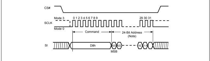
Note: Please note the address cycles above are based on 3-byte address mode. For 4-byte address mode, the address cycles will be increased.
