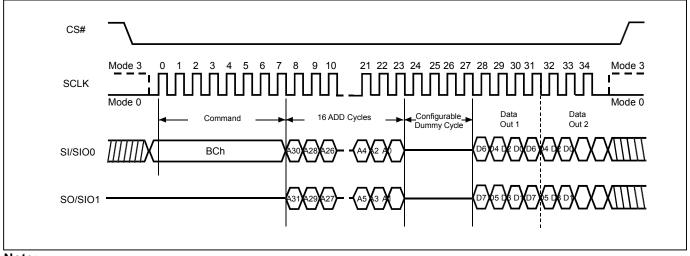
1. Configuration Dummy cycle numbers will be different depending on the bit6 & bit7 (DC0 & DC1) setting in configuration register.
