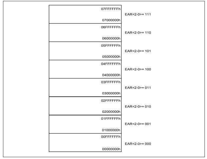
When under EAR mode, Read, Program, Erase operates in the selected segment by using 3-byte address mode.
