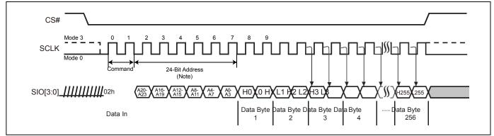
Note: Please note the address cycles above are based on 3-byte address mode. For 4-byte address mode, the address cycles will be increased.
