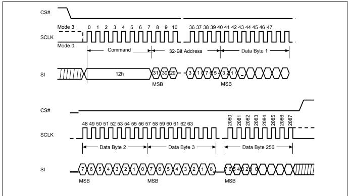
Figure 66. 4 x I/O Page Program (4PP4B) Sequence (SPI Mode only)
