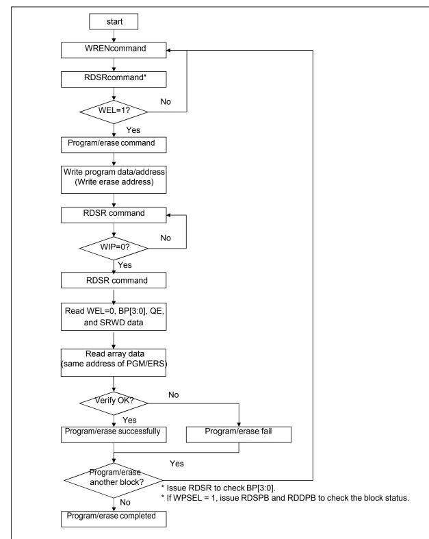
Figure 27. Program/Erase flow with read array data
