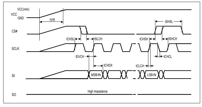
Figure 118. AC Timing at Device Power-Up
