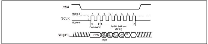
Note: Please note the address cycles above are based on 3-byte address mode. For 4-byte address mode, the address cycles will be increased.
