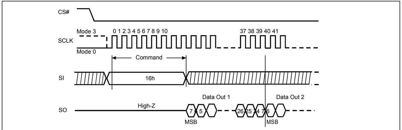
**Figure 76. Write Fast Boot Register (WRFBR) Sequence**
