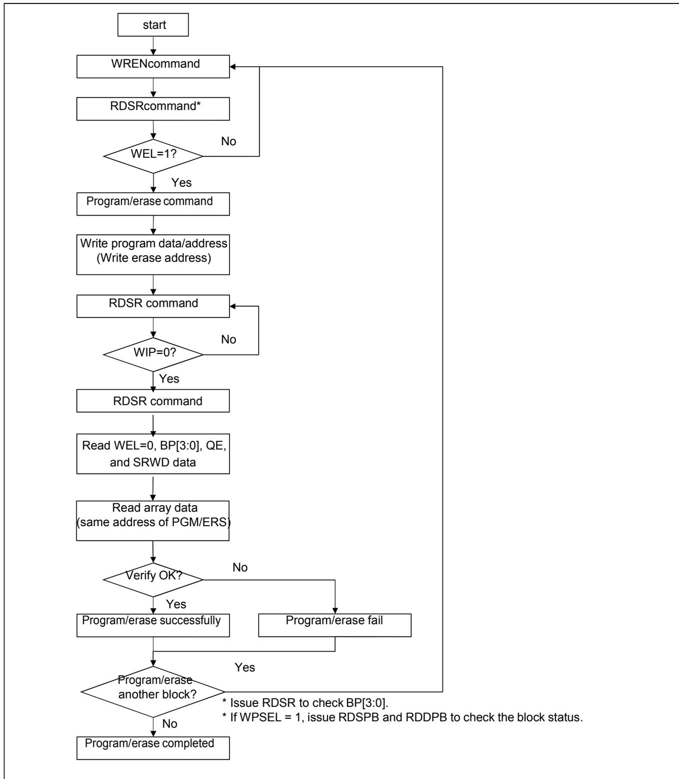
**Figure 28. Program/Erase flow without read array data (read P\_FAIL/E\_FAIL flag)**
