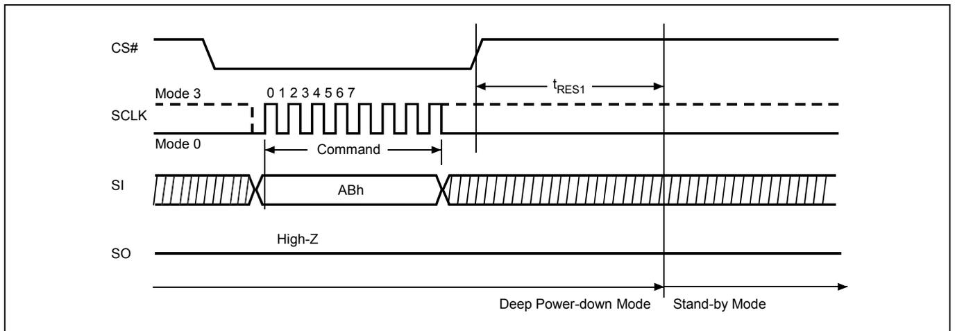
**Figure 21. Release from Deep Power-down (RDP) Sequence (QPI Mode)**
