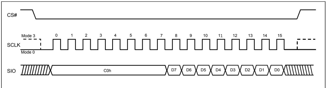
**Figure 72. Burst Read (QPI Mode)**
