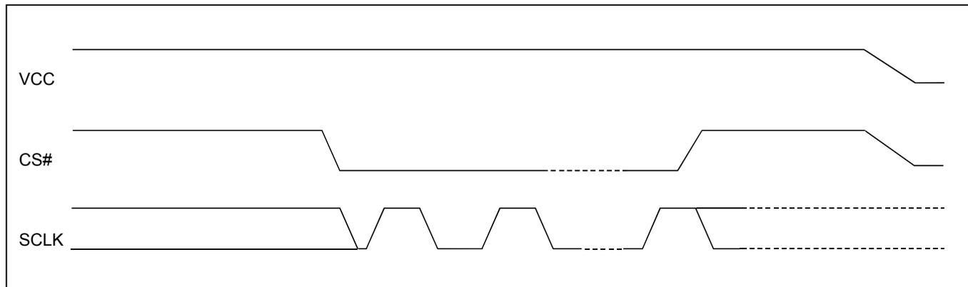
**Figure 120. Power-up Timing**
