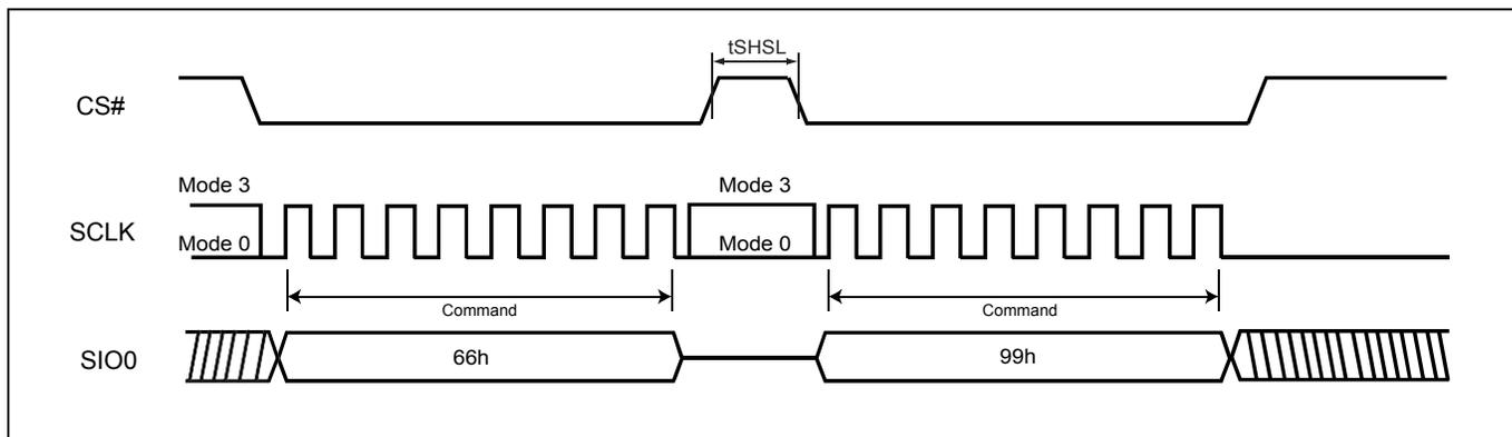
**Figure 110. Reset Sequence (QPI mode)**
