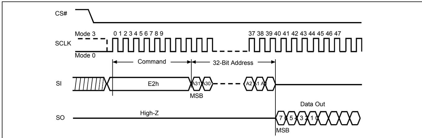
**Figure 98. SPB Erase (ESSPB) Sequence**
