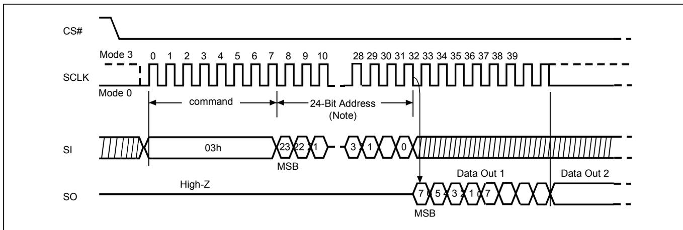
Note: Please note the address cycles above are based on 3-byte address mode. For 4-byte address mode, the address cycles will be increased.
