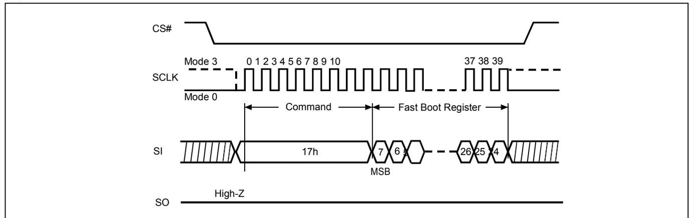
**Figure 77. Erase Fast Boot Register (ESFBR) Sequence**
