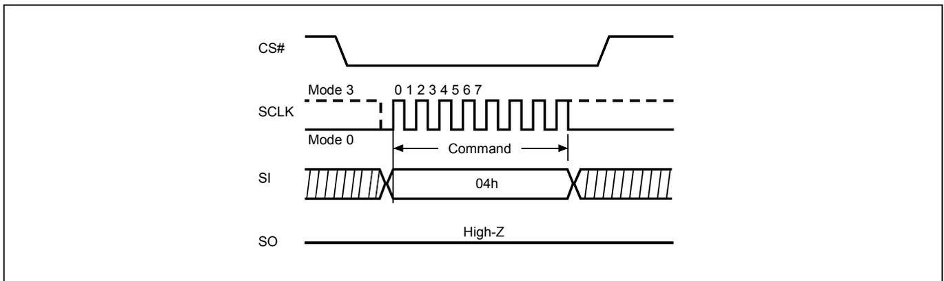
**Figure 14. Write Disable (WRDI) Sequence (QPI Mode)**
