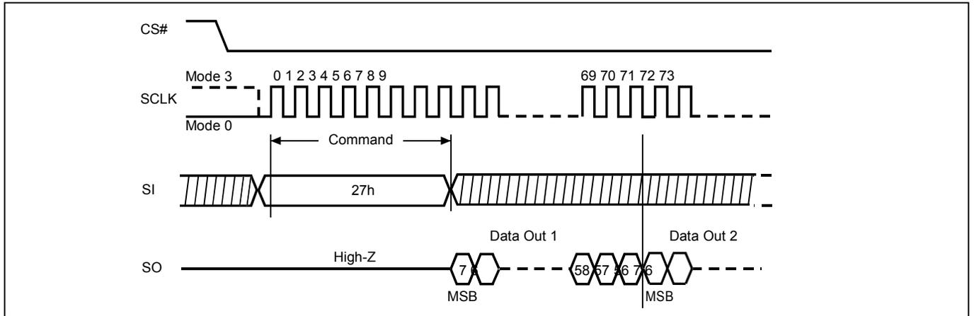
**Figure 103. Write Password Register (WRPASS) Sequence**
