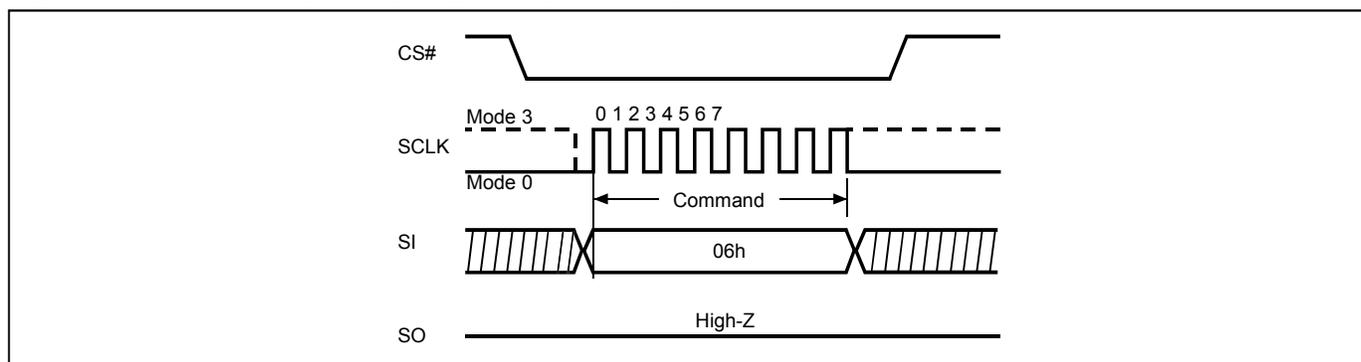
**Figure 12. Write Enable (WREN) Sequence (QPI Mode)**
