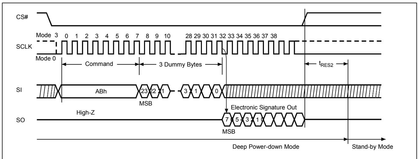
**Figure 19. Read Electronic Signature (RES) Sequence (QPI Mode)**
