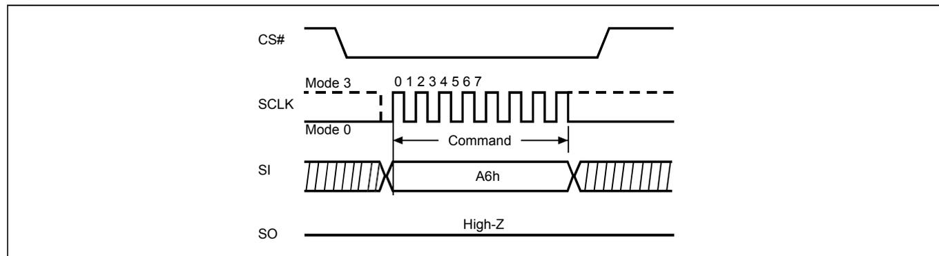
**Figure 96. Read SPB Lock Register (RDSPBLK) Sequence**
