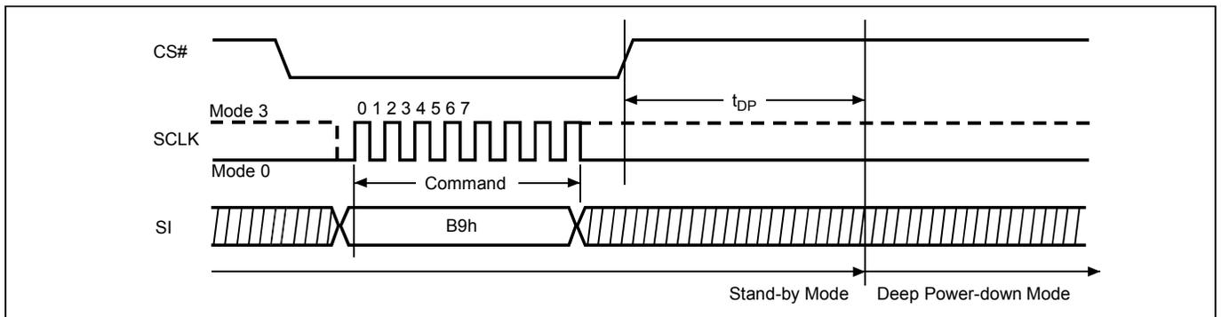
**Figure 90. Deep Power-down (DP) Sequence (QPI Mode)**
