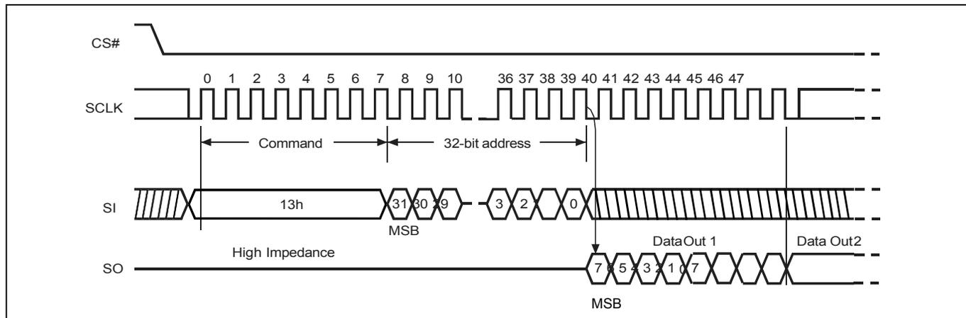
**Figure 55. Read Data Bytes at Higher Speed using 4-Byte Address Sequence (FASTREAD4B)**
