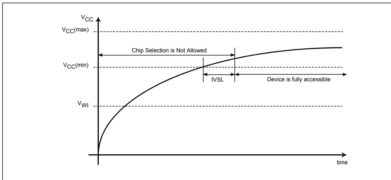
**Figure 121. Power Up/Down and Voltage Drop**
