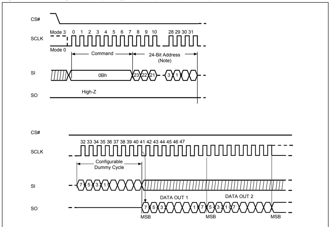
Note: Please note the address cycles above are based on 3-byte address mode. For 4-byte address mode, the address cycles will be increased.
