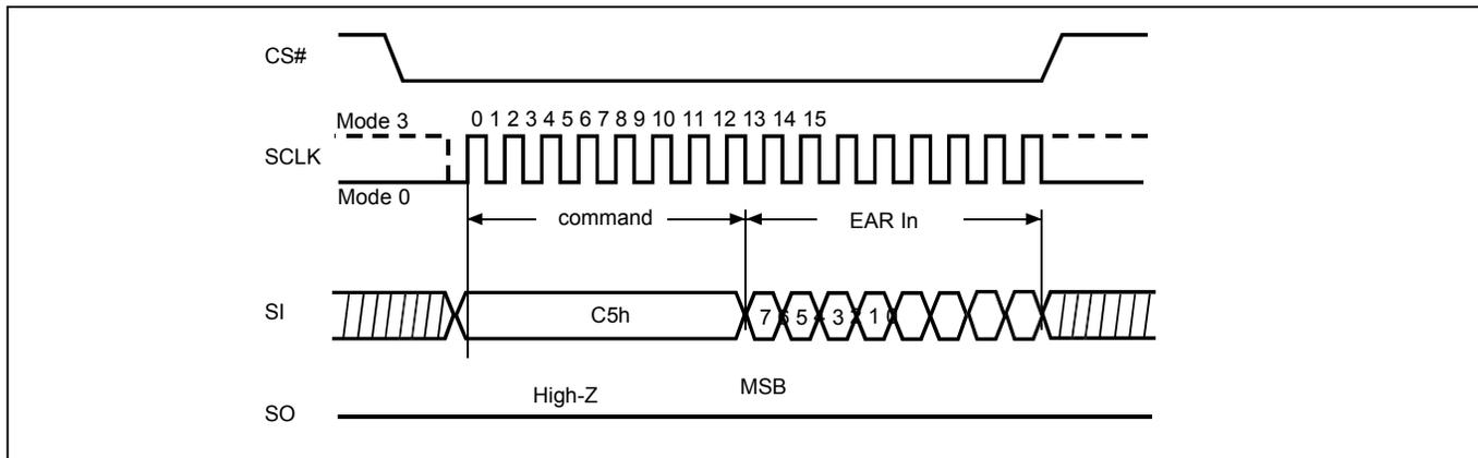
**Figure 6. Write EAR Register (WREAR) Sequence (QPI Mode)**
