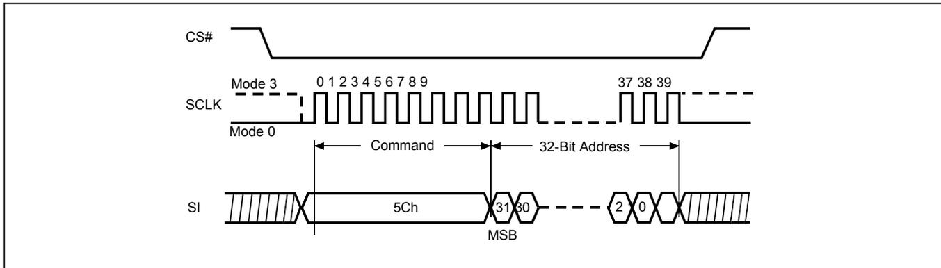
**Figure 64. Block Erase (BE4B) Sequence (SPI Mode)**
