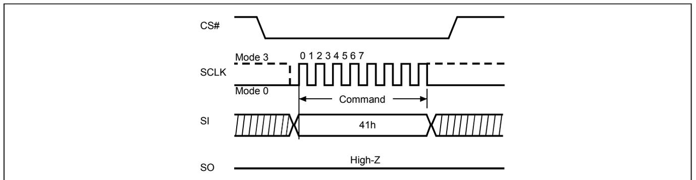
**Figure 16. Factory Mode Enable (FMEN) Sequence (QPI Mode)**
