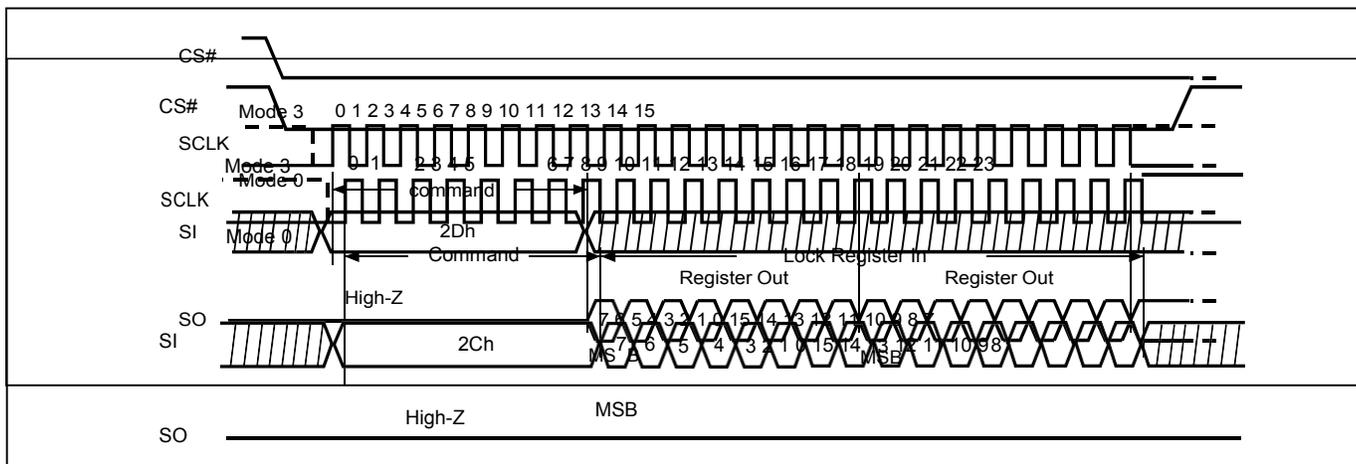
**Figure 94. Write Lock Register (WRLR) Sequence (SPI Mode)**
