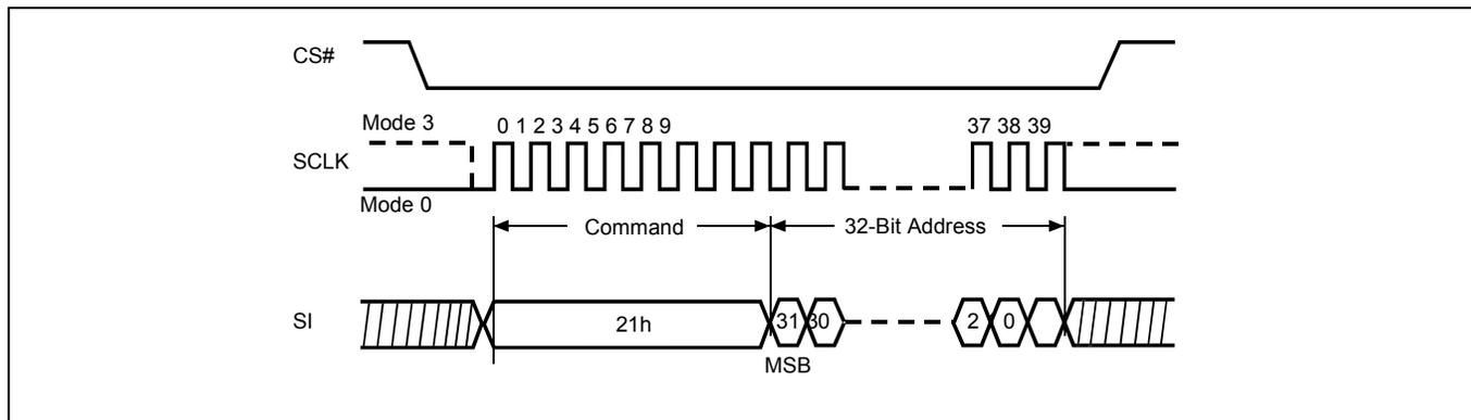
**Figure 63. Block Erase 32KB (BE32K4B) Sequence (SPI Mode)**
