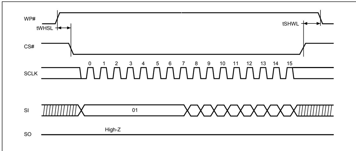
**Figure 11. Write Enable (WREN) Sequence (Command 06)**
