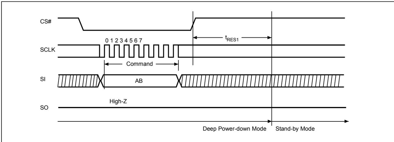
**Figure 35. Read Electronic Manufacturer & Device ID (REMS) Sequence (Command 90 or EF or DF or CF)**
