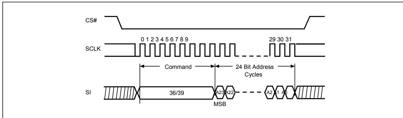
**Figure 38. Read Block Protection Lock Status (RDBLOCK) Sequence (Command 3C)**
