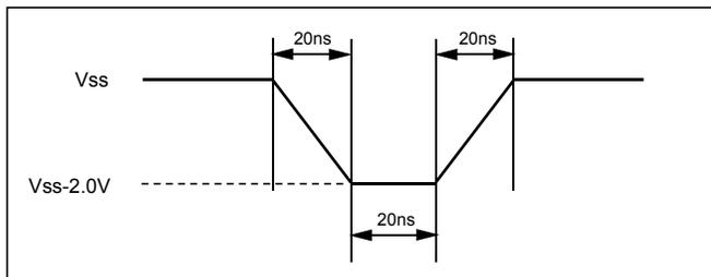
Figure 3. Maximum Positive Overshoot Waveform
