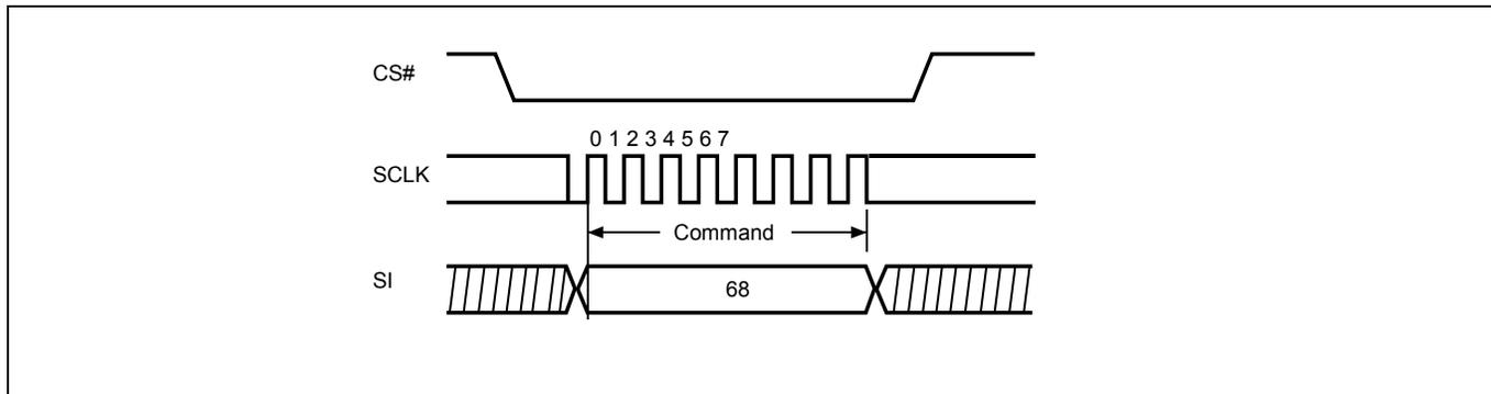
**Figure 37. Single Block Lock/Unlock Protection (SBLK/SBULK) Sequence (Command 36/39)**
