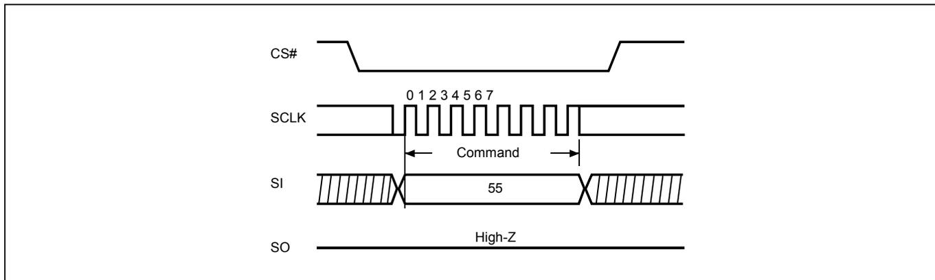
**Figure 31-2. Exit Parallel Mode (EXPLM) Sequence (Command 45)**
