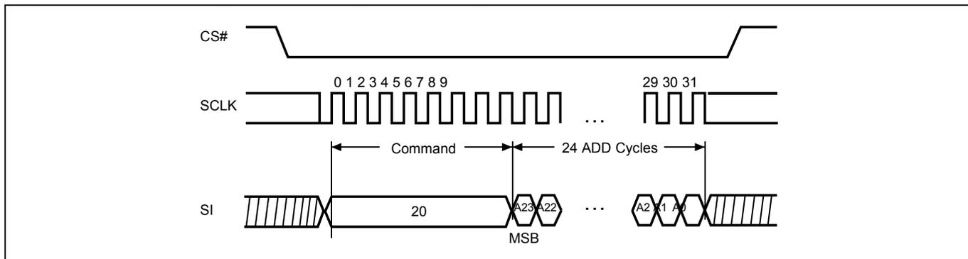
**Figure 26. Block Erase (BE/BE32K) Sequence (Command D8/52)**
