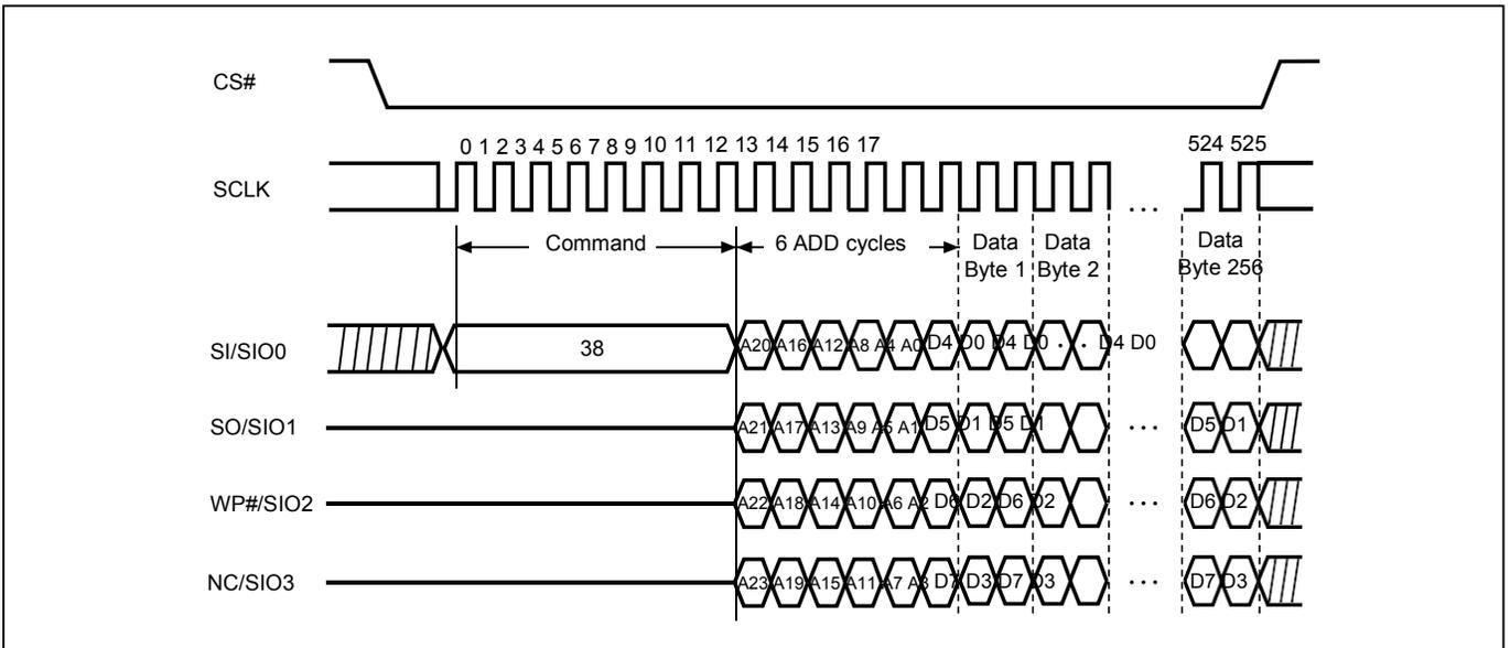
**Figure 30. Continuously Program (CP) Mode Sequence with Hardware Detection (Command AD)**
