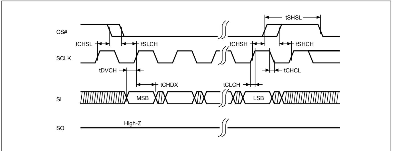
Figure 7. Output Timing
