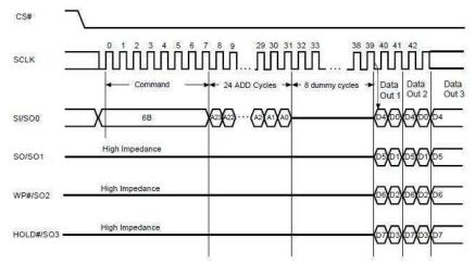
Figure 1: 4xI/O mode (1--1-4 mode) wavefrom
