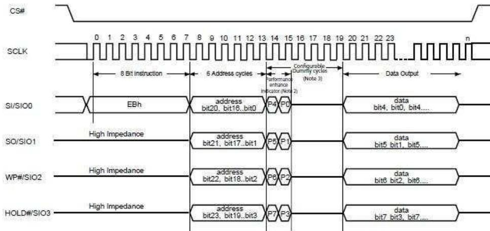
Figure2: Quad I/O mode ( 1-4-4 mode) waveform
