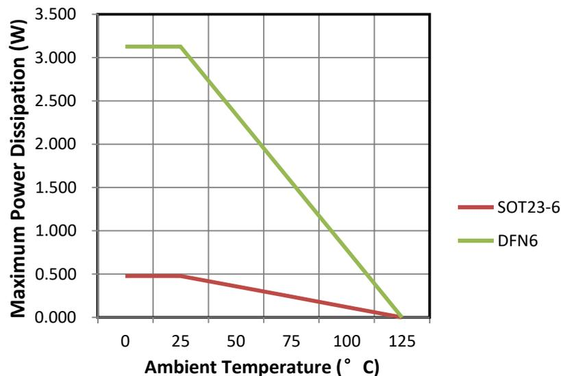
**Figure 3. Derating Curve of Maximum Power Dissipation**
