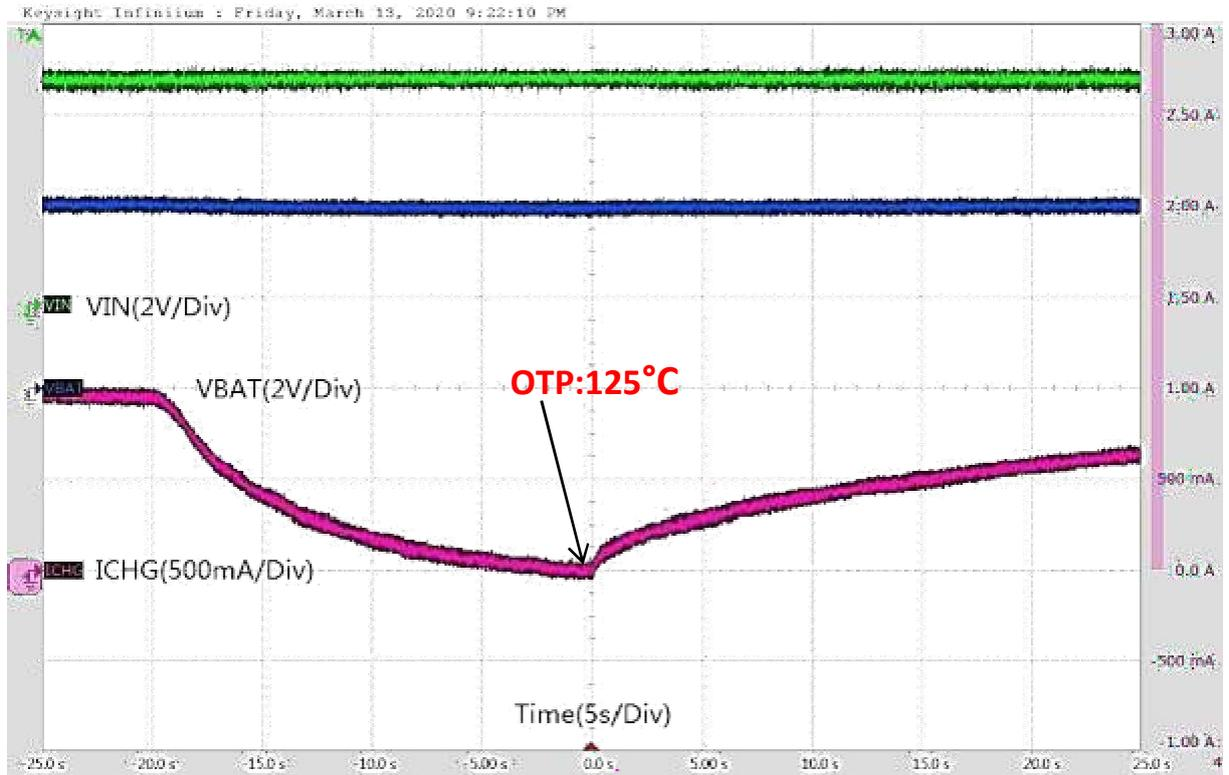
**Figure 4.Charging Temperature loop Profile**
