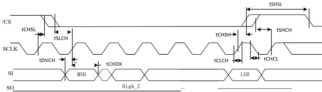
Figure 47. Output Timing
