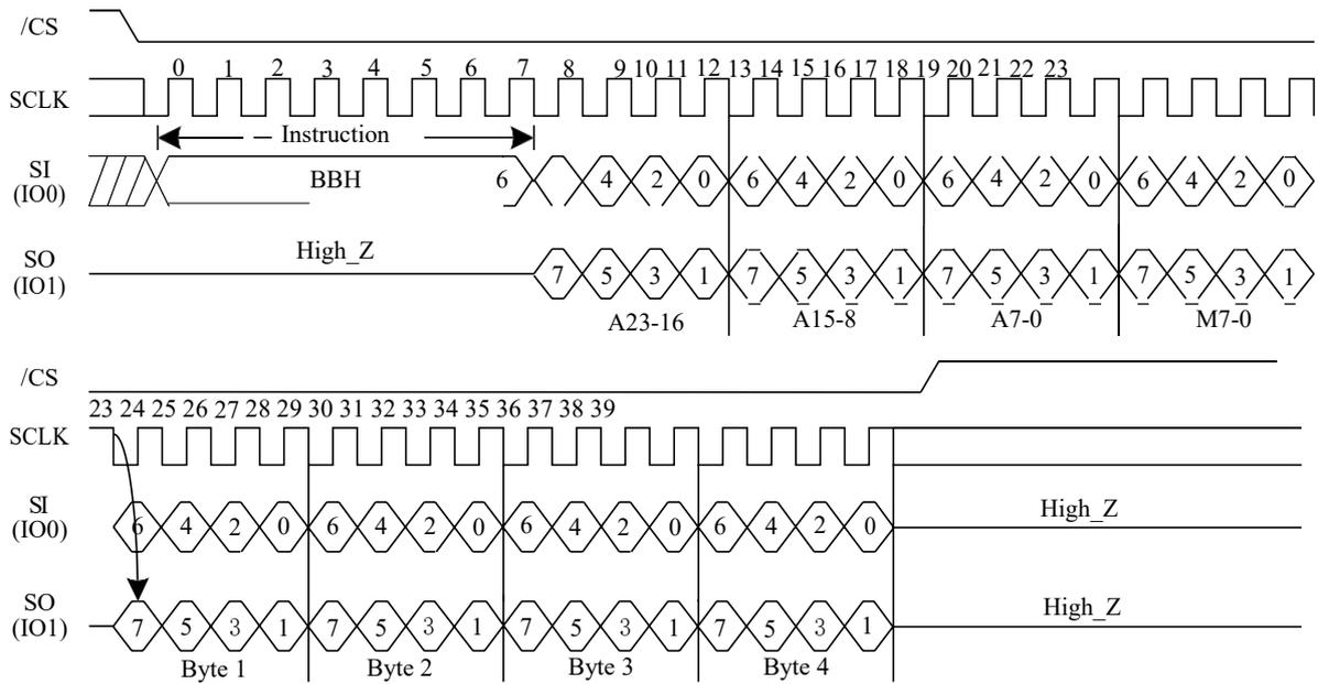
**Figure 14.b.** Dual I/O Fast Read Sequence Diagram (Previous command set (M5-4) =(1,0),SPI mode only)
