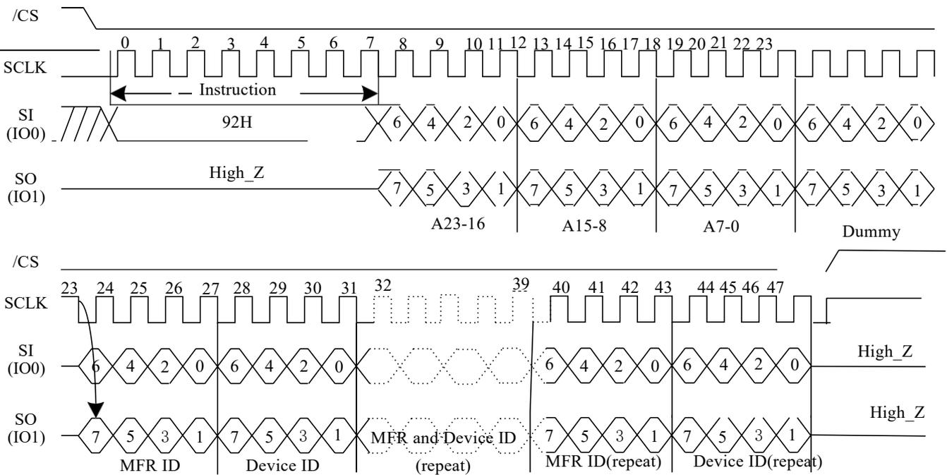
**7.3.3 Quad I/O Read Manufacture ID/ Device ID (94H)**
