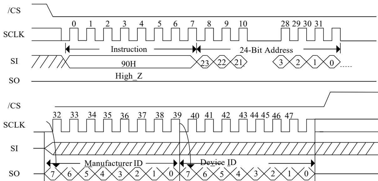
**7.3.2 Dual I/O Read Manufacture ID/ Device ID (92H)**
