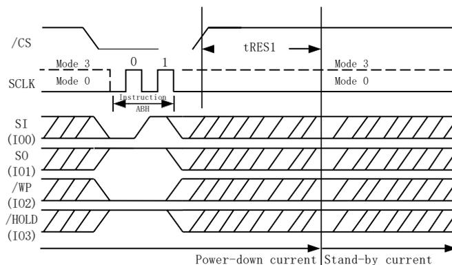
**Figure 26.c. Release Power-down / Device ID Instruction (SPI Mode)**
