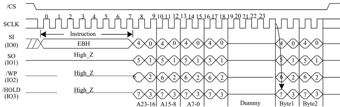
**Figure 15.b.** Quad I/O Fast Read Sequence Diagram (Previous command set (M5-4)=(1,0)), SPI mode only)
