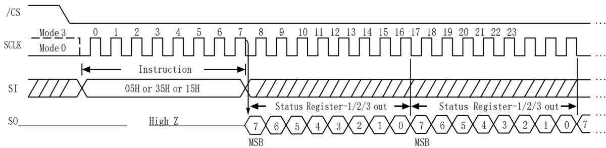
**Figure 7.b.** Read Status Register Sequence Diagram (QPI Mode)
