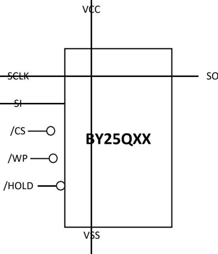
**Figure 2.** Pin Configuration SOP 208 mil
