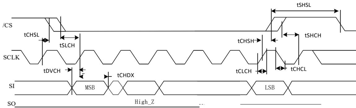
Figure 24. Output Timing
