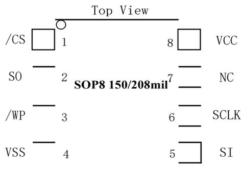
Figure 3. Pin Configuration DIP8L
