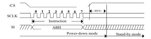
Figure 26.b. Release Power-down Instruction (QPI Mode)
