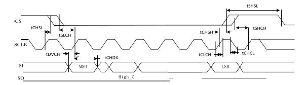
Figure 47. Output Timing
