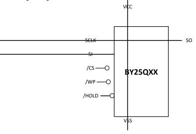
Figure 2. Pin Configuration SOP 208 mil
