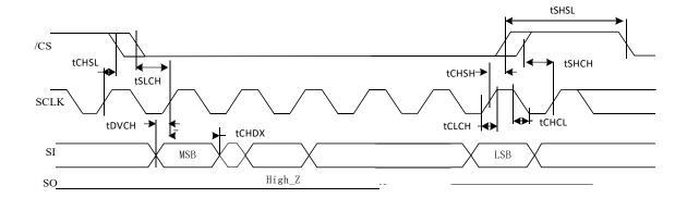
Figure 24. Output Timing
